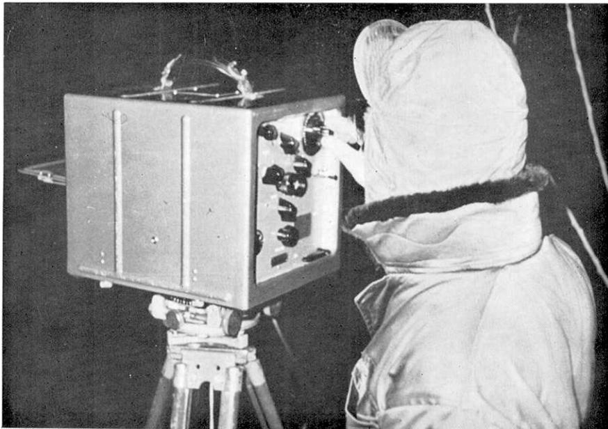
Fig. 10. Operation of a Geodimeter in the night.
