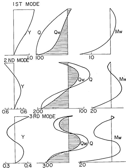
Fig. 5. Illustration of mode shapes, shears and moments.
