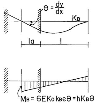
Fig. 4. Rigidity of boundary beams.
