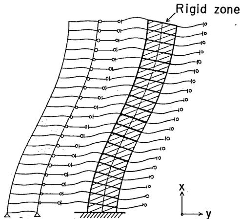
Fig. 2. Reduced vibratory system.
