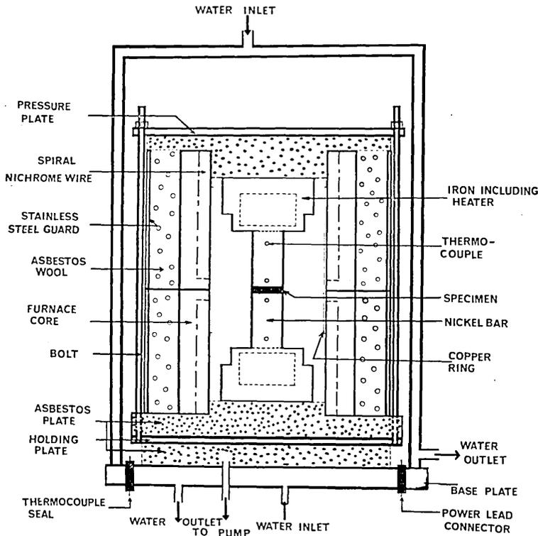
Fig. 2. Modified divided-bar device for measurement of thermal conductivity of rocks.
