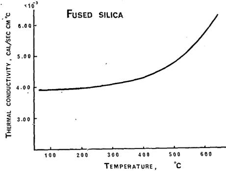
Fig. 6. Thermal conductivity of fused silica (after A. Goldsmith *et al.*).
