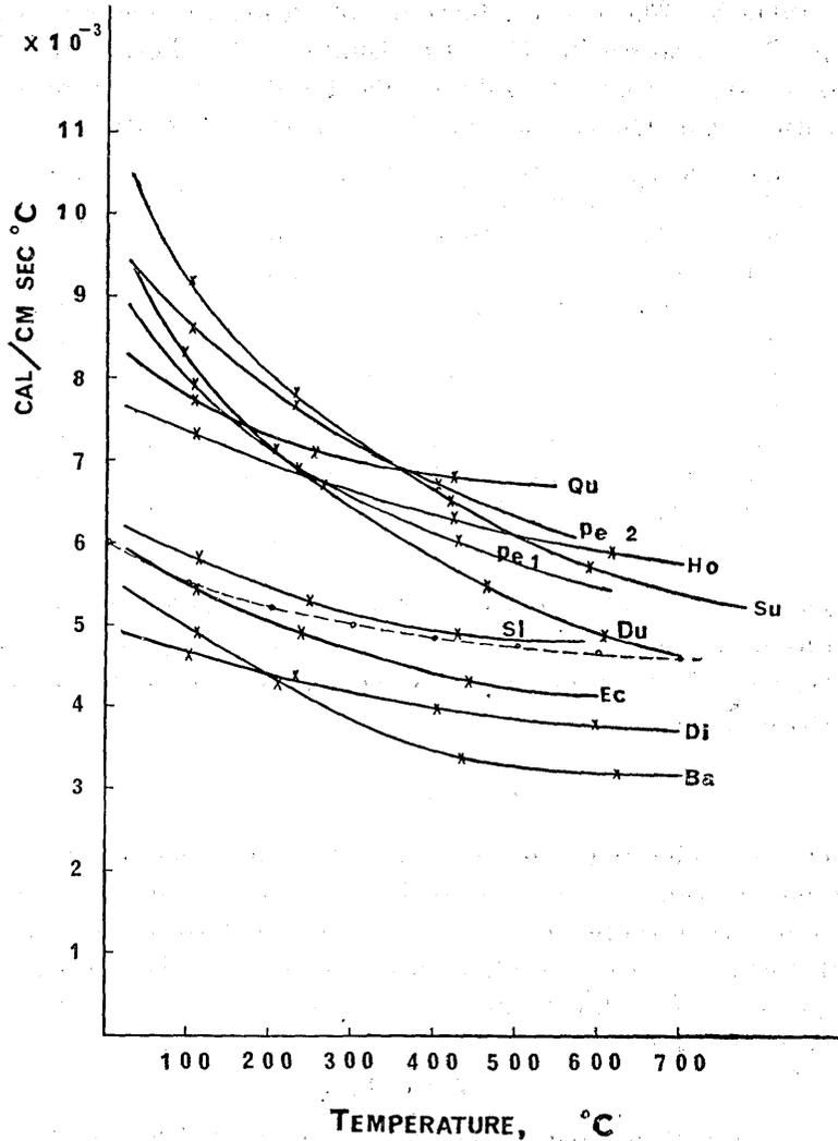
Fig. 8. Thermal conductivity of rocks.
