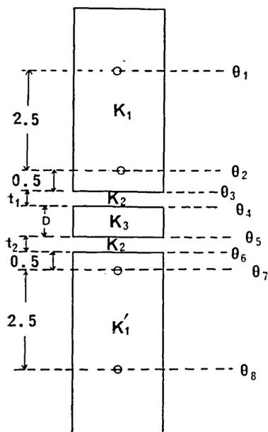
Fig. 4. "Constant temperature difference" divided-bar apparatus.
