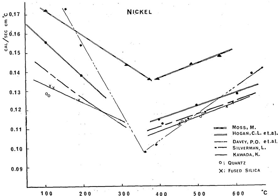
Fig. 7. Thermal conductivity of nickel.
