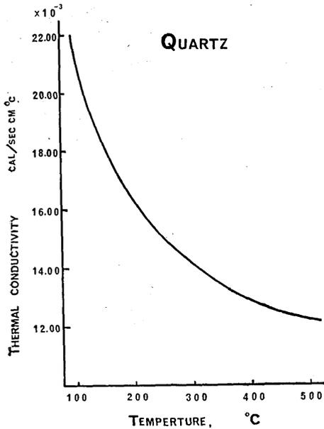
Fig. 5. Thermal conductivity of quartz (after A. Goldsmith *et al.*).
