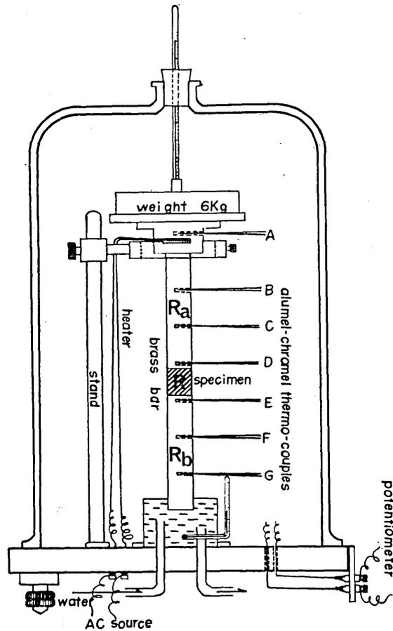
Fig. 1. Divided-bar device for measurement of thermal conductivity of rocks.
