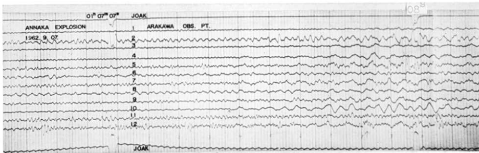
Fig. 5-25. Seismogram obtained at Arakawa for Annaka explosion.
