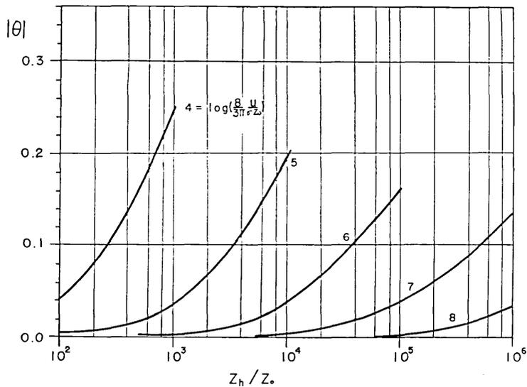
Fig. 3b. Phase  $\theta$  of the frictional coefficient  $C$  as a function of  $z_h/z_0$  for the oscillating turbulent flow over a rough surface.
