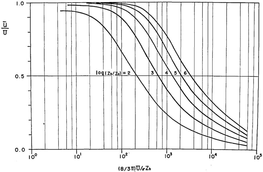
Fig. 4a. The ratio of the depth-mean velocity  $\hat{u}$  to the velocity  $U$  for the case of no friction as a function of  $U/(\sigma z_h)$  with  $z_h/z_0$  as a parameter.
