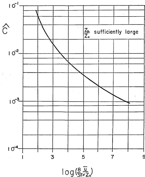
Fig. 3 c. Amplitude  $\hat{C}$  of the frictional coefficient  $C$  as a function of  $\bar{u}/(\sigma z_0)$  for sufficiently large values of  $z_h/z_0$ .
