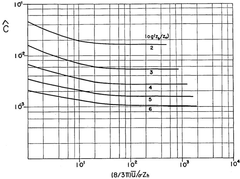
Fig. 2a. Amplitude  $\hat{C}$  of the frictional coefficient  $C$  as a function of  $\bar{u}/(\sigma z_h)$  for the oscillating turbulent flow over a rough surface.
