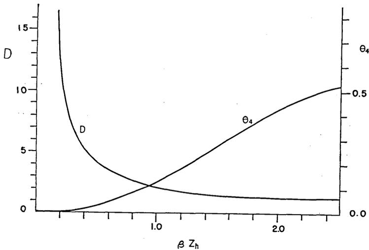
Fig. 9.  $D$  and  $\theta_4$  as a function of  $\beta z_h$  for the laminar oscillating flow.
