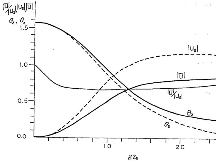
Fig. 8. Amplitudes (non-dimensional) and phases of the mean velocity and surface velocity, and the ratio of the mean velocity to the surface velocity as a function of  $\beta z_h$  for the laminar oscillating flow.
