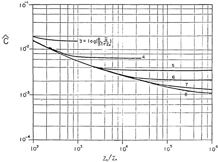
Fig. 3a. Amplitude  $\hat{C}$  of the frictional  $C$  as a function of  $z_h/z_0$  for the oscillating turbulent flow over a rough surface.
