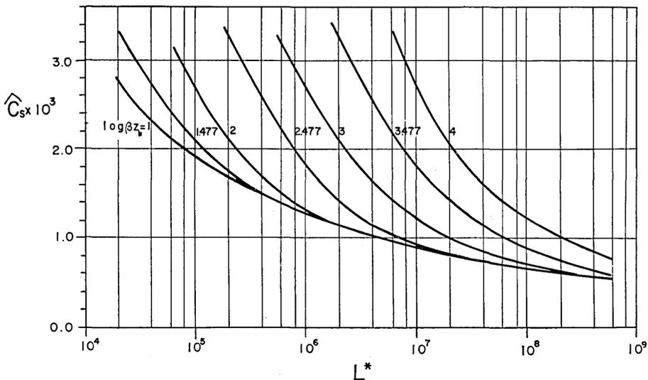
Fig. 5a. Amplitude  $\hat{C}_s$  of the frictional coefficient  $C_s$  as a function of a Reynolds number  $L^*$  for the oscillating turbulent flow over a smooth surface.
