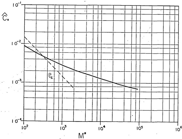
Fig. 6 a. Amplitude  $\hat{C}_s$  of the frictional coefficient  $C_s$  as a function of a Reynolds number  $M^*$  for large values of  $\beta z_k (> 0.6\sqrt{L})$ . Broken line indicates the amplitude of the laminar frictional coefficient  $C_l$ .
