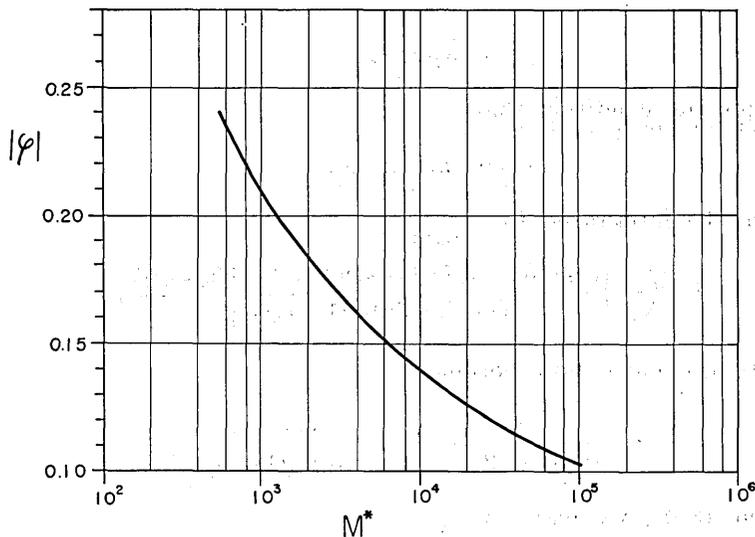
Fig. 6b. Phase  $\varphi$  of the frictional coefficient  $C_s$  as a function of a Reynolds number  $M^*$  for large values of  $\beta z_h (> 0.6\sqrt{L})$ .
