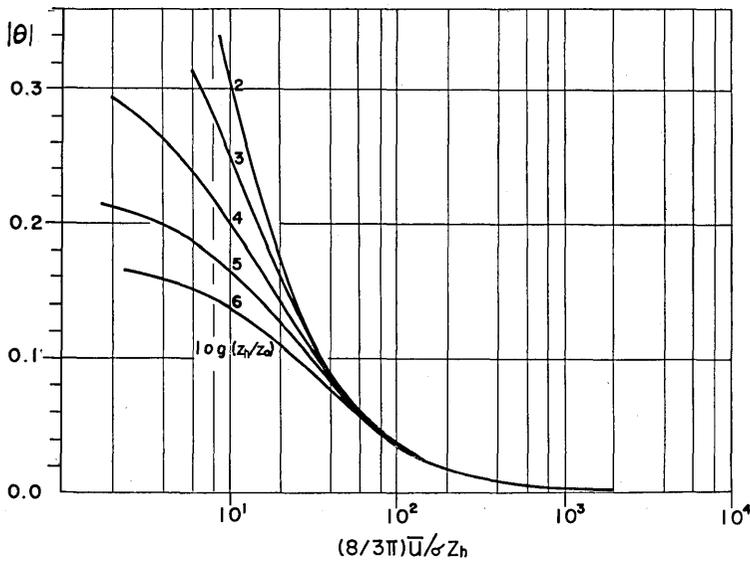
Fig. 2b. Phase  $\theta$  of the frictional coefficient  $C$  as a function of  $\bar{u}/(\sigma z_h)$  for the oscillating turbulent flow over a rough surface.
