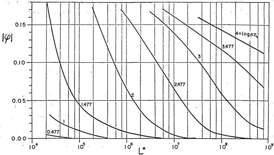
Fig. 5 b. Phase  $\varphi$  of the frictional coefficient  $C_s$  as a function of a Reynolds number  $L^*$  for the oscillating turbulent flow over a smooth surface.
