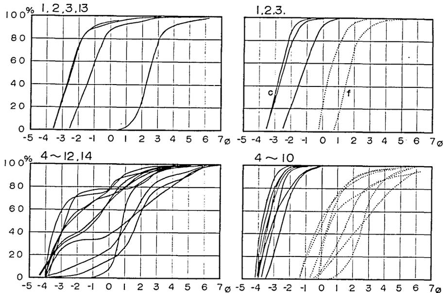
Fig. 5. Size distribution curves of ash fall deposits from outbursts on Nov. 10 and 11, 1958. Upper: the ash fall from the outburst on Nov. 11. Lower: the ash fall from the outburst on Nov. 10. The left diagrams show the whole curve of each specimen, and the right diagrams show the separate curves of two units with different coarseness in each specimen, i. e., c (solid curve) represents the coarser unit and f (dotted curve) represents the finer unit.
