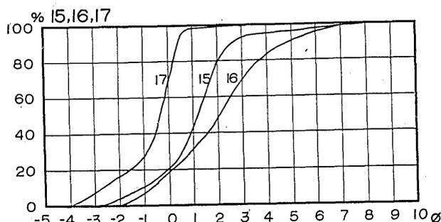
Fig. 9. Size distribution curves of ash fall deposits from outbursts which occurred in Dec., 1958, and on Apr. 14, 1959.
