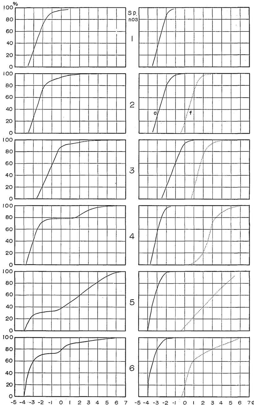
Fig. 6a. Size distribution curves of ash fall deposits from outbursts on Nov. 10 and 11, 1958, showing the curve of each specimen separately. The right diagrams show separate curves of two units with different coarseness in each specimen, as those in Fig. 5.
