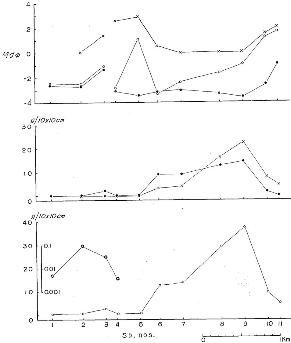
Fig. 8. Variation of coarseness ( $Md\phi$  value) and density of ash fall deposits from outbursts on Nov. 10 and 11, 1958, along the road running from south to north on the eastern slope of Mt. Asama. The localities of specimens are shown in Fig. 1. Open circles represent the value of the whole specimen, solid circles represent the value of the coarser unit, crosses represent the value of the finer unit, and double circles represent the value of pumice.
