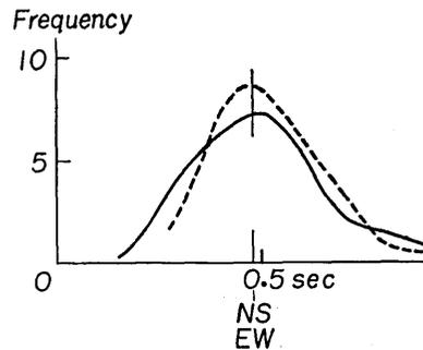
Fig. 5. Period distribution curve of the earthquake motion obtained at the roof floor of N Building.
