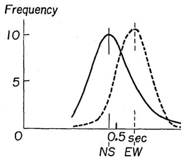
Fig. 6. Period distribution curve of the earthquake motion obtained at the roof floor of I Building.
