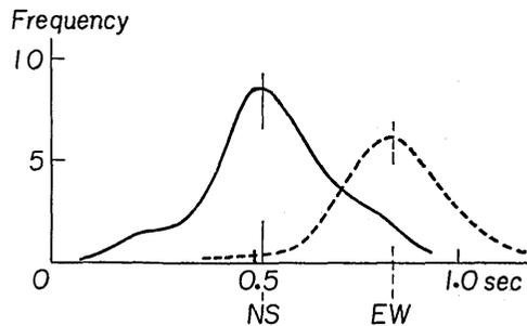
Fig. 3. Period distribution curve of the earthquake motion obtained at the twelfth floor of K Building.
