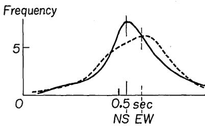
Fig. 4. Period distribution curve of the earthquake motion obtained at the roof floor of S Building.
