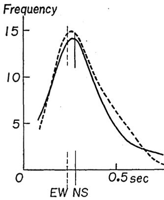
Fig. 2. Period distribution curve of the earthquake motion obtained at the roof floor of M Building.
