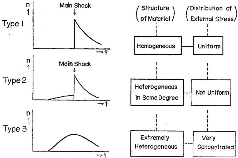
Fig. 2. Three types of the successive occurrence of the elastic shocks accompanying fractures and their relations to the structures of materials and the applied stresses.
