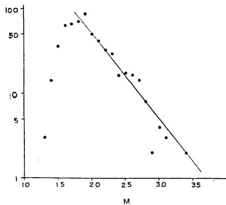
Fig. 12. Frequency distribution of magnitudes of earthquakes belonging to the sequences "A" and "B".  $b=1.0$
