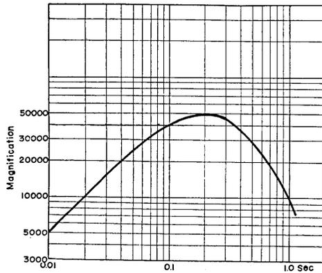
Fig. 2. Magnification vs. period curves of the "HES 1-0.2" seismograph at the Kurobe IV Dam. Seismograph constants are as follows:
