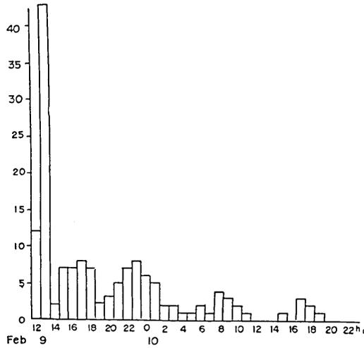
Fig. 4. Hourly frequencies of earthquakes recorded at the Kurobe IV Dam with p-s intervals between 2.0 and 4.0 seconds. Main part of the sequence "A".
