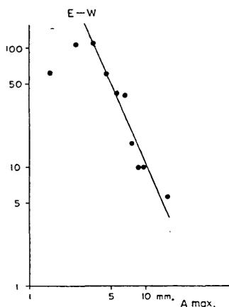
Fig. 10. Frequency distribution of Maximum trace amplitudes.  $m=2.2$
