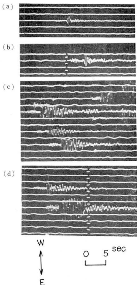
Fig. 7. Typical "HES 1-0.2" seismograms recorded at the Kurobe IV Dam.
