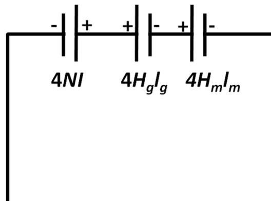
Figure 4.10: Equivalent magnetic circuit considering one magnetic circuit.
