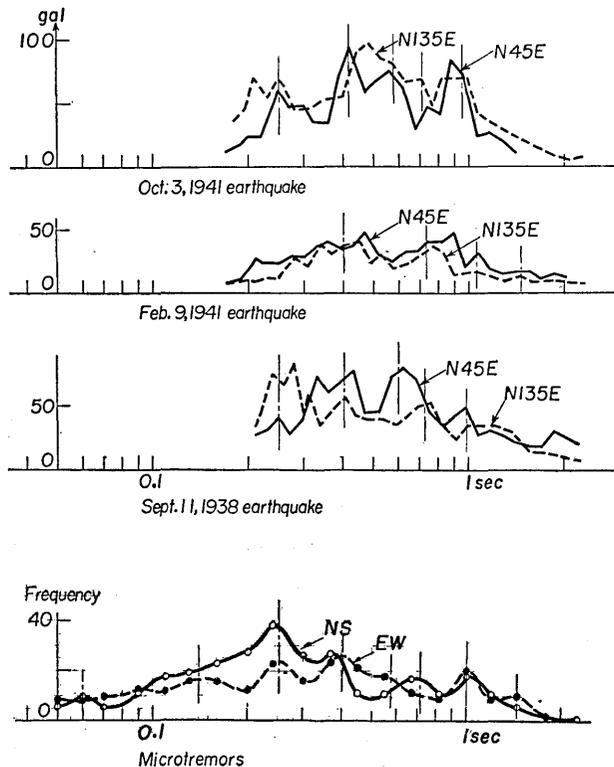
Fig. 2. The relation between the acceleration spectra of three earthquakes observed at Ferndale, California, U.S.A. and the period distribution curve of microtremors at the same place. The vertical strips of chain line represent the maximum frequent periods of microtremors.
