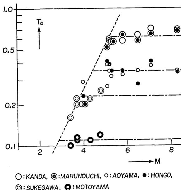
Fig. 1. The relation between the predominant period of earthquake motions and the magnitude of earthquake,  $M$ .
