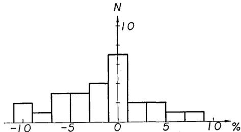
Fig. 6. Relation between the number of measurements and the percentage residual of the mean periods to the resonance periods.
