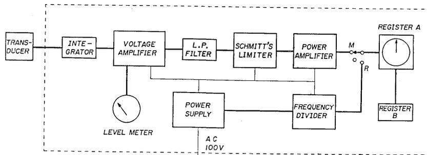
Fig. 3. Block diagram showing the constitution of the natural period meter.
