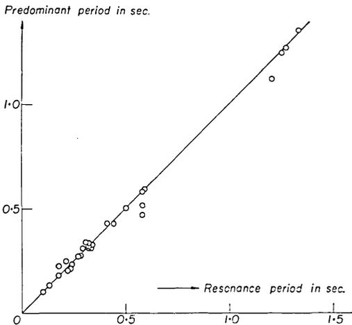
Fig. 2. Relation between the predominant period in normal times and the resonance period obtained from the vibration experiments of the actual buildings.
