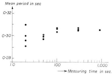
Fig. 4. Relation of the mean period to the measuring time.
