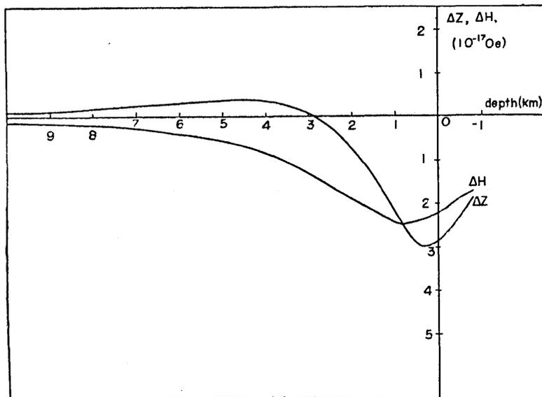
Fig. 7. The anomalous values of horizontal and vertical components at Nomashi caused by a unit magnetic dipole with positive polarity at various depths right below the crater.
