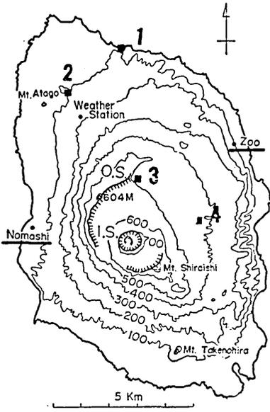
Fig. 1. Topographical map of Oshima Island. Underlined are the locations of magnetic observatories. Square dots 1, 2, 3 and 4 are the bore-holes. The temperature distributions in the holes are shown in Figs. 8, 9, 10 and 11 respectively.
