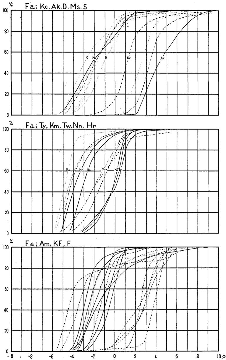
Fig. 4 Cumulative curves of the particle size distribution of pyroclastic fall deposits.
