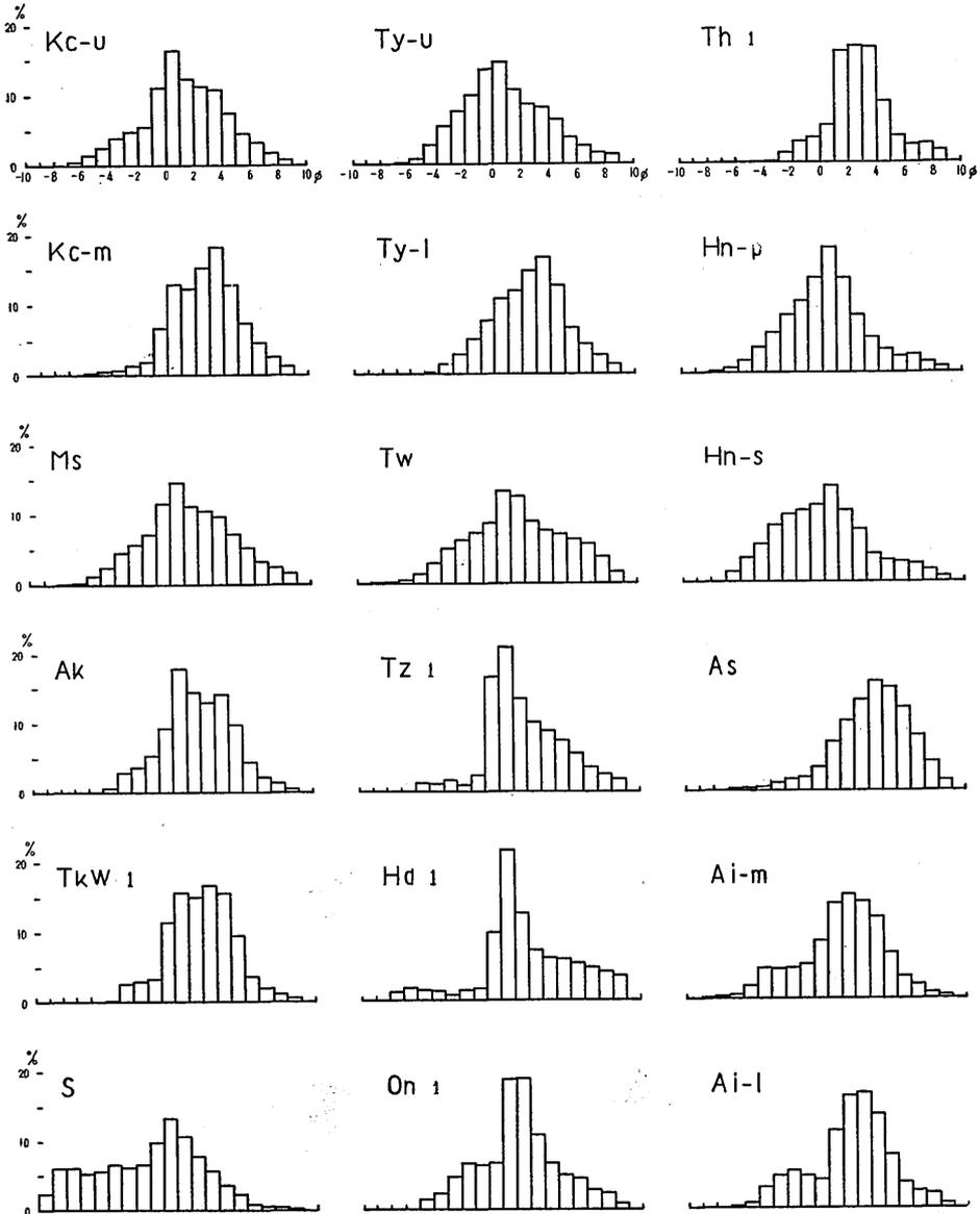
Fig. 11. Histograms of particle size distribution of the pyroclastic flow deposits. One which represents the individual result of only one sample is noted by its sample number. The others represent the average results of several samples.
