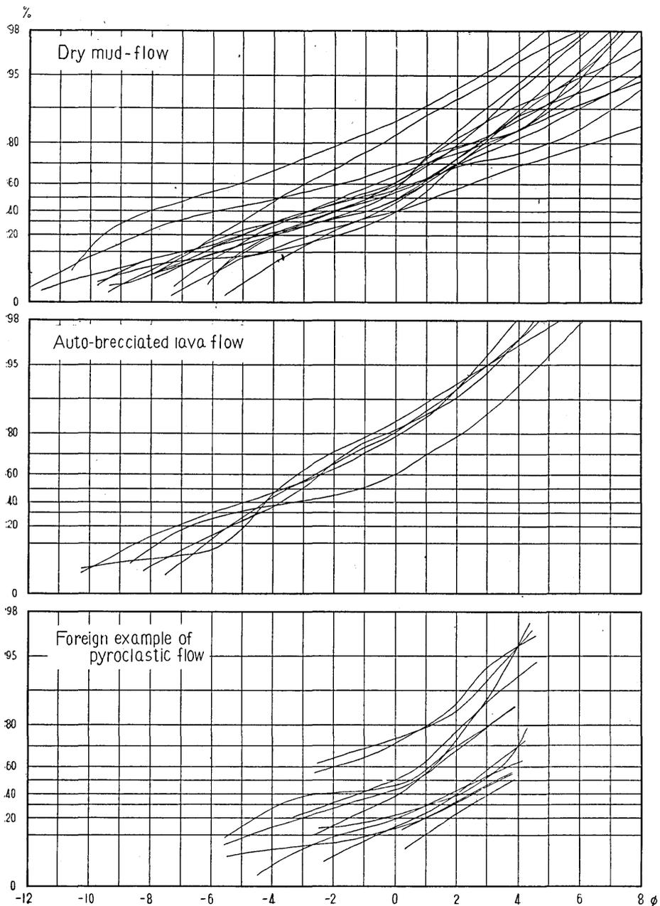
Fig. 10. Cumulative curves plotted on Rosin law paper. Upper: dry mud-flows, middle: auto-brecciated lava flows, lower: foreign examples of pyroclastic flows. Every line represents a curve of each individual sample.
