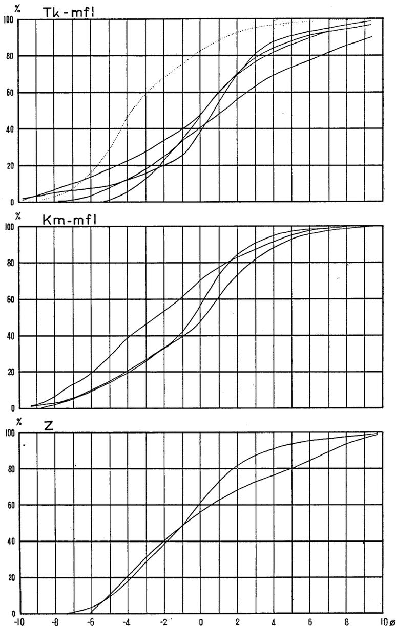
Fig. 5a. Cumulative curves of the particle size distribution of dry mud-flow deposits. Upper: the Tokachidake Volcano (solid line: May 24th, 1926, dotted line: Sept. 3rd, 1926), middle: the Komagatake Volcano, lower: the Zao Volcano.
