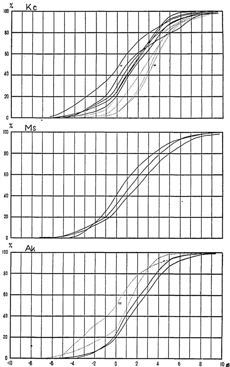
Fig. 3. Cumulative curves of the particle size distribution of pyroclastic flow deposits.
