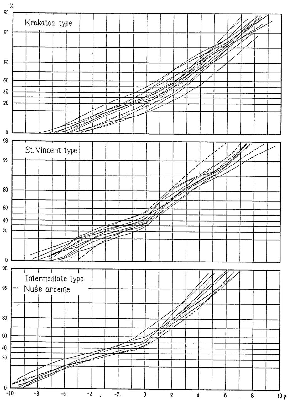
Fig. 9. Cumulative curves of the pyroclastic flow deposits plotted on Rosin law paper. The explanation of the curves is the same as in Fig. 8.
