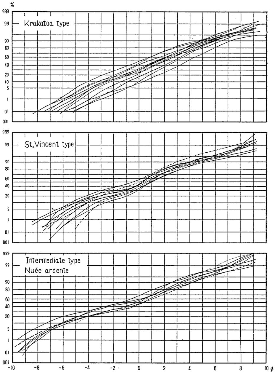
Fig. 8. Cumulative curves of the pyroclastic flow deposits plotted on normal probability paper. Solid lines are average curves of samples in a single unit of pyroclastic flow. Dotted lines are curves of one sample. Each curve represents one unit of flow. Broken lines in the middle figure represent the variety having an intermediate nature between the St. Vincent type ash-flows and dry mud-flows. A broken line in the lower figure is a curve of a nuée ardente.
