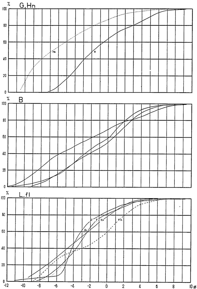
Fig. 5b. Cumulative curves of the particle size distribution of dry mud-flow deposits and auto-brecciated lava flows. Upper: mud-flows of the Gassan and Hakone Volcanoes, middle: the 1888 Mud-flow of the Bantai Volcano, lower: autobrecciated lava flows.
