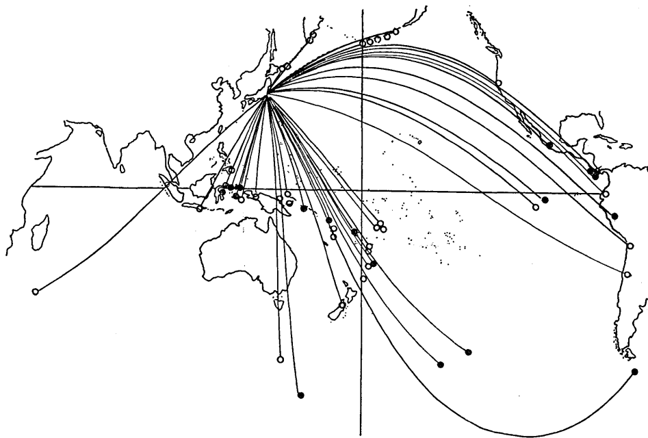
Fig. 1. Epicenters and travelling paths of Rayleigh waves across the oceanic basin. The epicenters newly added and of the previous ones are represented by black and white circles respectively.
