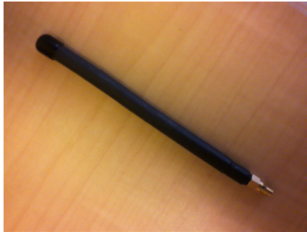
図 5.3: Dipole antenna (vertically set to surface at experiment)
