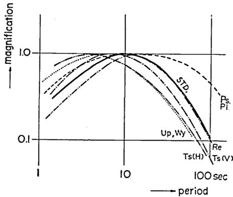
Fig. 6. Frequency response curves of seismographs.
