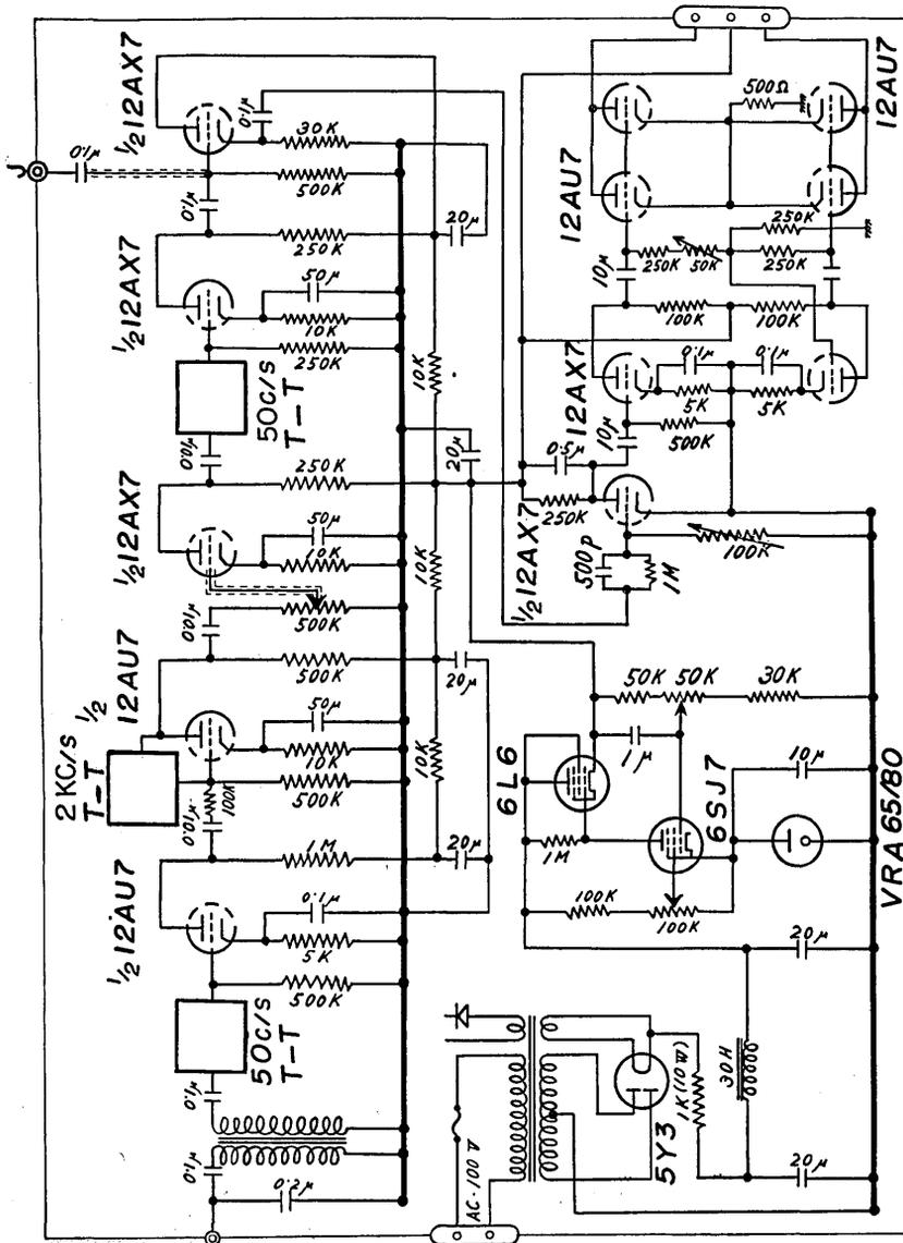
Fig. 2. Electric circuits of amplifier 2, power supply, mixing part and power amplifier.
