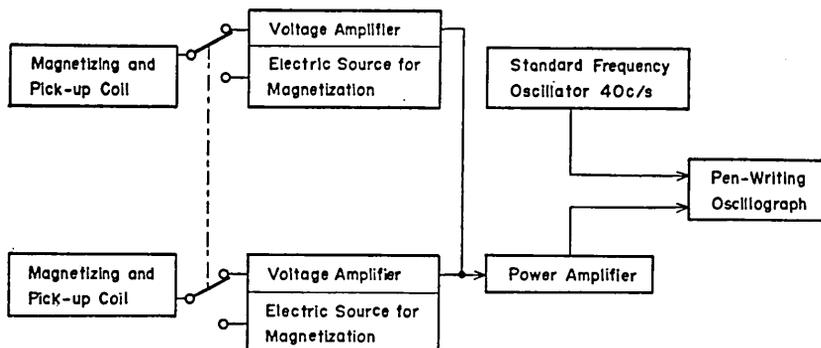
Fig. 1. Block-diagram of the differential proton magnetometer.
