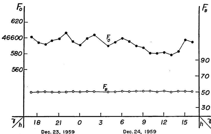
Fig. 5. Results of the observation by the station-use proton magnetometer ( $F_0$ ) and the differential proton magnetometer ( $F_B$ ) on Dec. 23 and 24, 1959.
