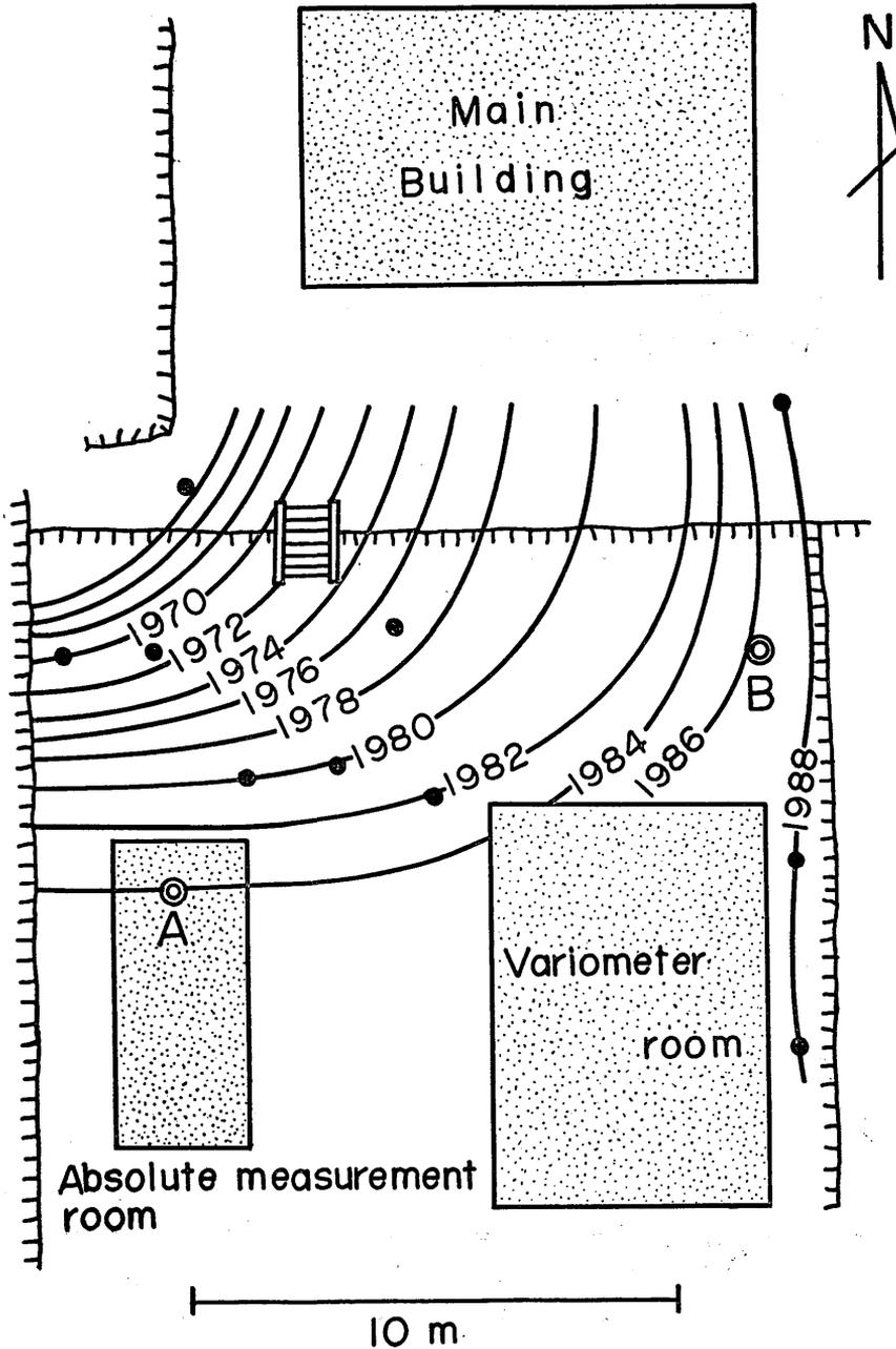
Fig. 3. The distribution of the proton precession frequencies (c/s) in the Oshima Geophysical Observatory. The detecting coils of the differential proton magnetometer are set at points A and B. The coil at A is also used for the routine observations of the total geomagnetic field by the station-use proton magnetometer.
