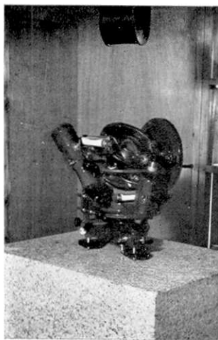
Fig. 1. The detector coil hung above the GSI magnetometer in the absolute measurement room of Oshima Geophysical Observatory.
