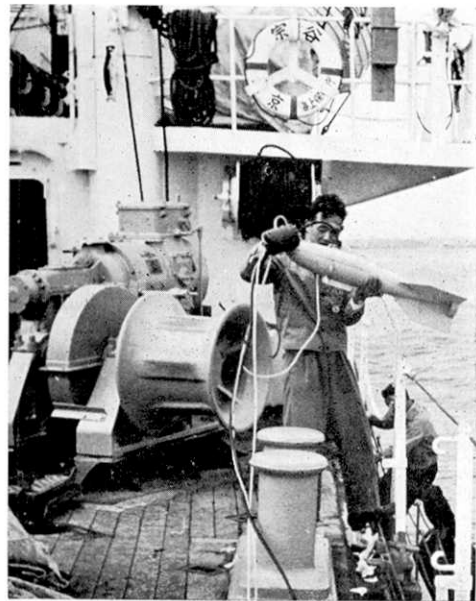
Fig. 5. The stream-lined case for the detector coil.
