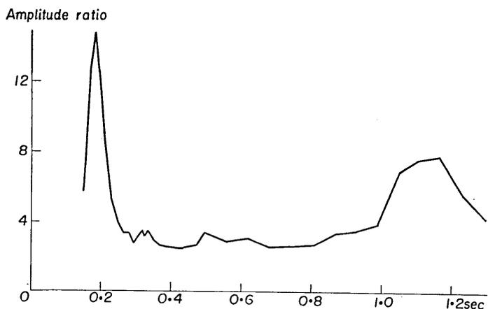
Fig. 6. Amplitude ratio of the ground surface to the 300 m depth at Hitachi Mine. Earthquake number: 378.
