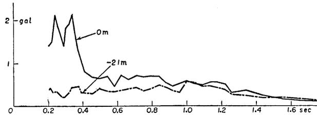
Fig. 60. Acceleration spectra of earthquake No. 56 at place (A) in Tokai-mura.
