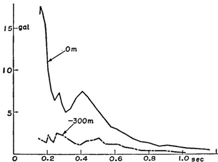
Fig. 30. Acceleration spectra of earthquake No. 797 at Hitachi Mine.
