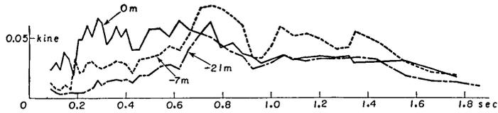
Fig. 83. Velocity spectra of earthquake No. 19 at place (B) in Tokai-mura.
