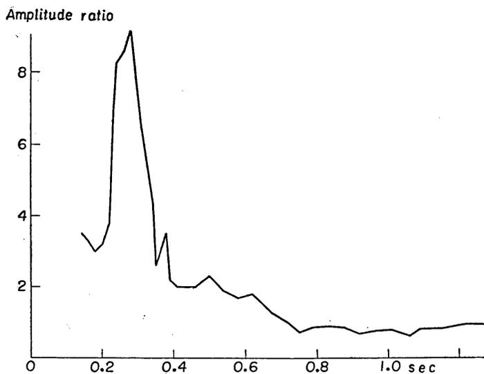
Fig. 64. The ratio of the amplitude on the ground to the one 21 m depth at place (A) in Tokai-mura. Earthquake number: 41.
