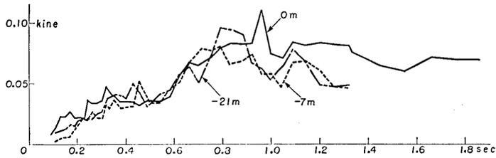
Fig. 84. Velocity spectra of earthquake No. 24 at place (B) in Tokai-mura.
