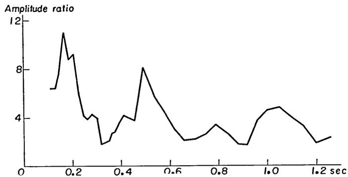
Fig. 10. Amplitude ratio of the ground surface to the 300 m depth at Hitachi Mine. Earthquake number: 828.
