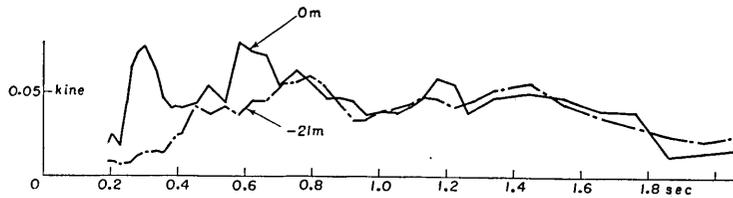
Fig. 49. Velocity spectra of earthquake No. 53 at place (A) in Tokai-mura.
