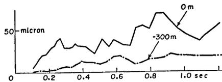
Fig. 18. Displacement spectra of earthquake No. 837 at Hitachi Mine.
