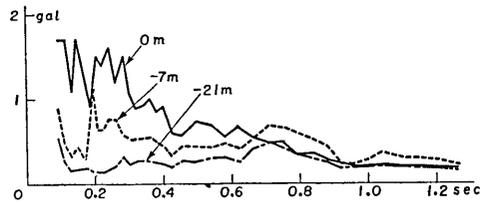
Fig. 90. Acceleration spectra of earthquake No. 19 at place (B) in Tokai-mura.
