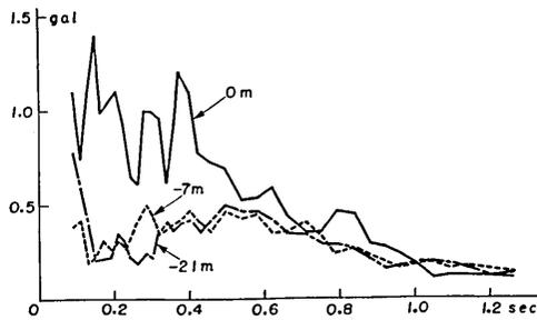
Fig. 92. Acceleration spectra of earthquake No. 27 at place (B) in Tokai-mura.
