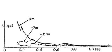
Fig. 86. Acceleration spectra of earthquake No. 3 at place (B) in Tokai-mura.
