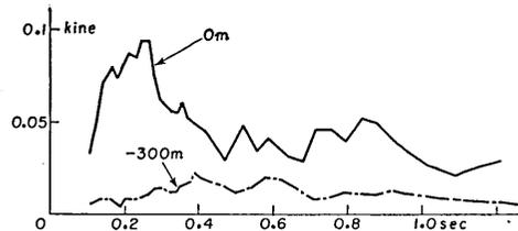
Fig. 25. Velocity spectra of earthquake No. 837 at Hitachi Mine.
