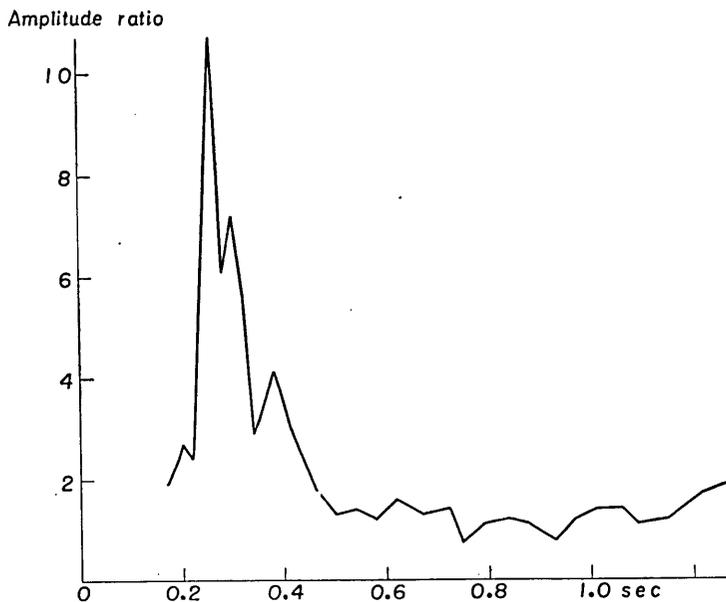
Fig. 70. The ratio of the amplitude on the ground to the one 21 m depth at place (A) in Tokai-mura. Earthquake number: 63.
