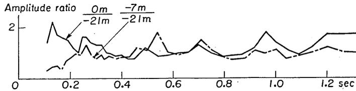
Fig. 98. Amplitude ratio corresponding to each period at place (B) in Tokai-mura. Earthquake number: 24.
