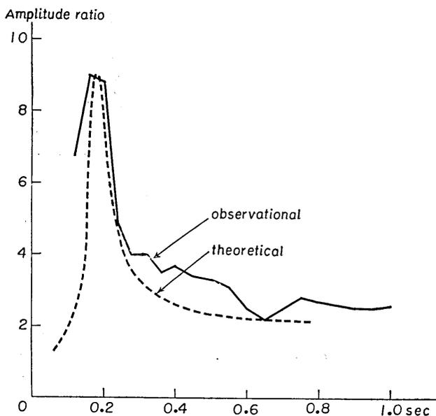
Fig. 101. Average amplitude ratio of 0 m to -300 m at Hitachi Mine.
