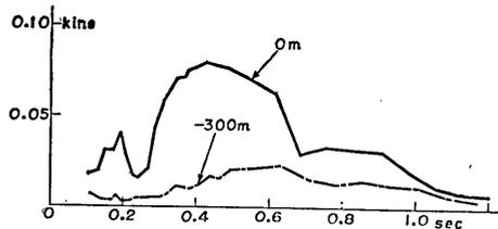
Fig. 19. Velocity spectra of earthquake No. 200 at Hitachi Mine.
