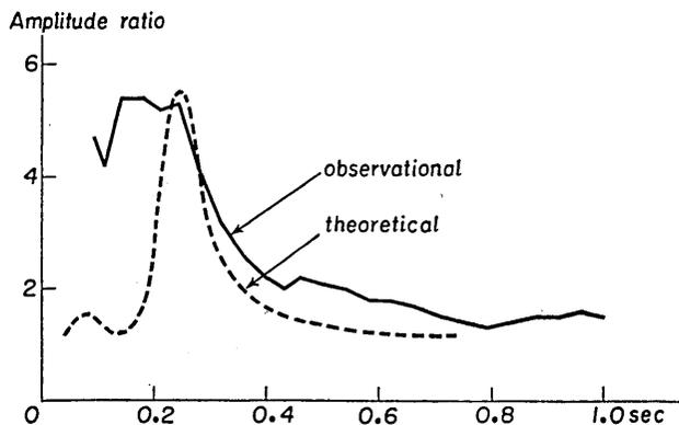
Fig. 103. Average amplitude ratio of 0 m to -21 m at place (B) in Tokai-mura.
