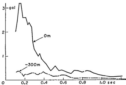
Fig. 32. Acceleration spectra of earthquake No. 837 at Hitachi Mine.
