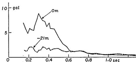
Fig. 54. Acceleration spectra of No. 39 earthquake at place (A) in Tokai-mura.
