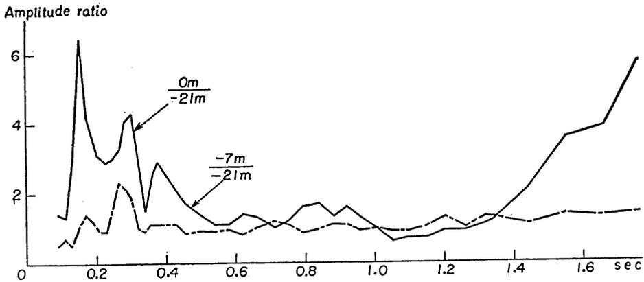
Fig. 99. Amplitude ratio corresponding to each period at place (B) in Tokai-mura. Earthquake number: 27.
