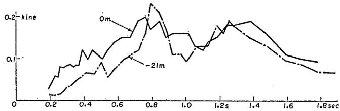
Fig. 48. Velocity spectra of earthquake No. 50 at place (A) in Tokai-mura.
