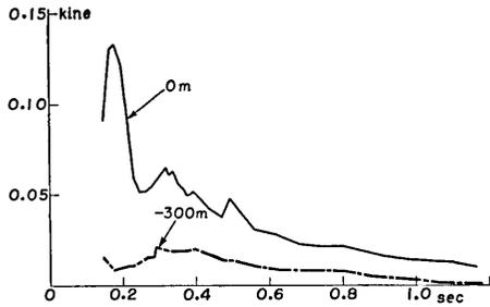
Fig. 20. Velocity spectra of earthquake No. 378 at Hitachi Mine.
