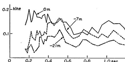
Fig. 82. Velocity spectra of earthquake No. 20 at place (B) in Tokai-mura.
