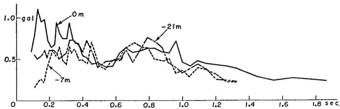
Fig. 91. Acceleration spectra of earthquake No. 24 at place (B) in Tokai-mura.
