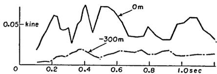
Fig. 24. Velocity spectra of earthquake No. 828 at Hitachi Mine.
