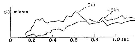
Fig. 37. Displacement spectra of earthquake No. 41 at place (A) in Tokai-mura.
