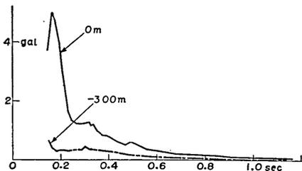
Fig. 27. Acceleration spectra of earthquake No. 378 at Hitachi Mine.
