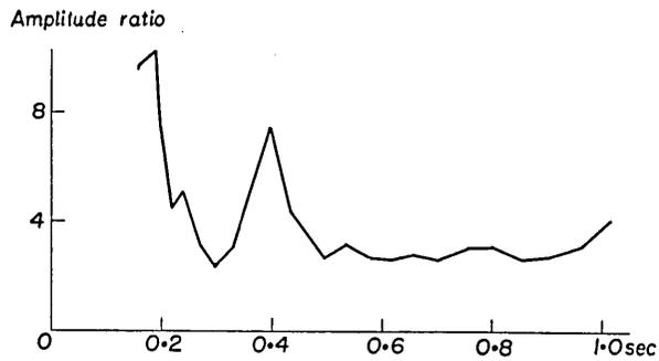
Fig. 9. Amplitude ratio of the ground surface to the 300 m depth at Hitachi Mine. Earthquake number: 797.
