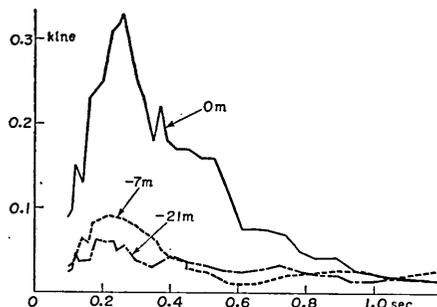
Fig. 80. Velocity spectra of earthquake No. 5 at place (B) in Tokai-mura.
