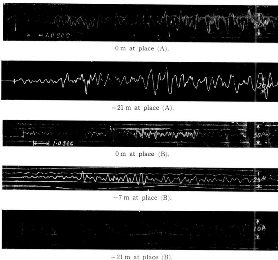
Fig. 34. Representative seismograms observed at Tokai-mura.
