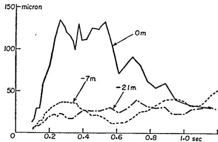
Fig. 73. Displacement spectra of earthquake No. 5 at place (B) in Tokai-mura.
