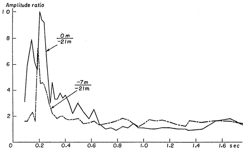
Fig. 96. Amplitude ratio corresponding to each period at place (B) in Tokai-mura. Earthquake number: 19.
