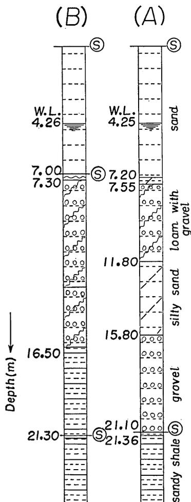
Fig. 33. Subsoil conditions of places (A) and (B) in Tokai-mura as detected by boring.
