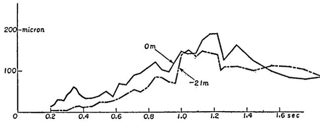
Fig. 42. Displacement spectra of earthquake No. 56 at place (A) in Tokai-mura.
