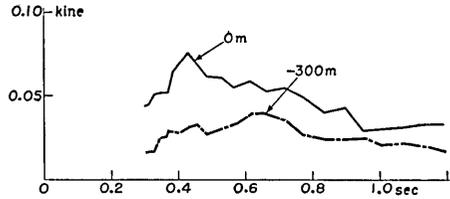
Fig. 21. Velocity spectra of earthquake No. 428 at Hitachi Mine.
