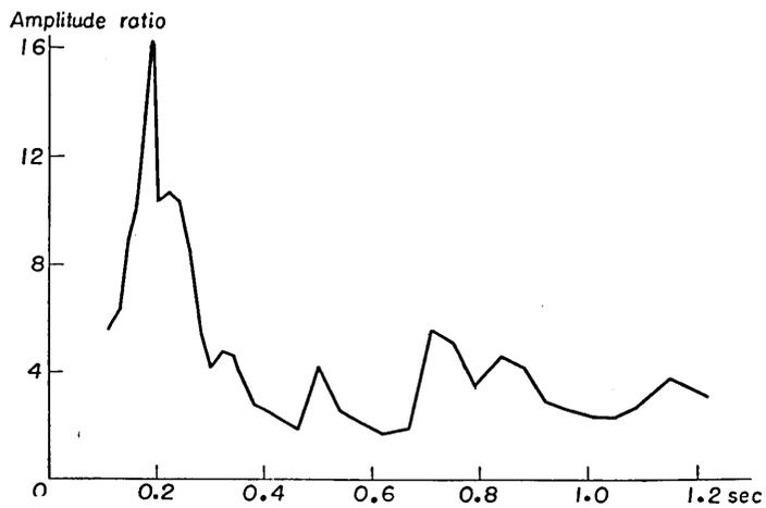
Fig. 11. Amplitude ratio of the ground surface to the 300 m depth at Hitachi Mine. Earthquake number: 837.
