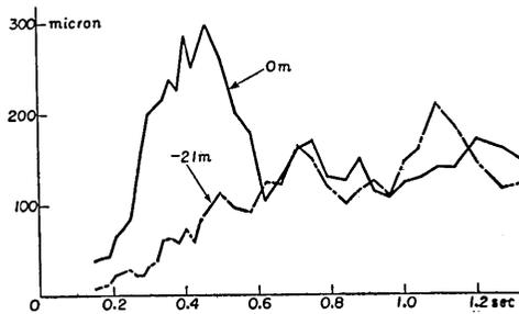
Fig. 36. Displacement spectra of earthquake No. 39 at place (A) in Tokai-mura.
