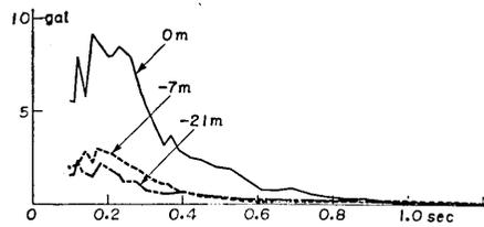
Fig. 87. Acceleration spectra of earthquake No. 5 at place (B) in Tokai-mura.
