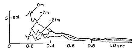
Fig. 89. Acceleration spectra of earthquake No. 20 at place (B) in Tokai-mura.
