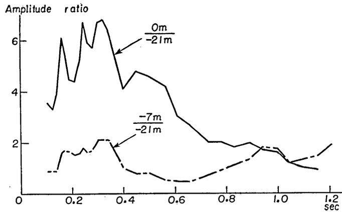
Fig. 94. Amplitude ratio corresponding to each period at place (B) in Tokai-mura. Earthquake number: 5.
