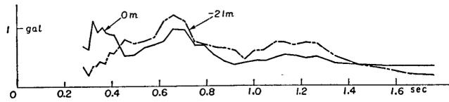
Fig. 59. Acceleration spectra of earthquake No. 55 at place (A) in Tokai-mura.
