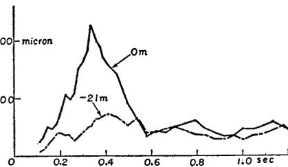
Fig. 44. Displacement spectra of earthquake No. 48 at place (A) in Tokai-mura.
