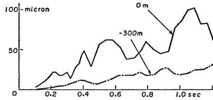
Fig. 17. Displacement spectra of earthquake No. 828 at Hitachi Mine.
