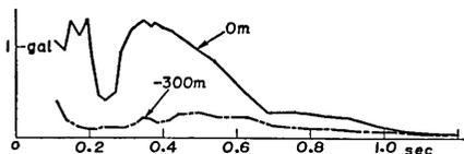
Fig. 26. Acceleration spectra of earthquake No. 200 at Hitachi Mine.
