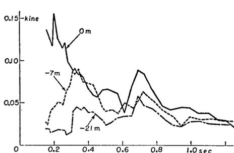
Fig. 79. Velocity spectra of earthquake No. 3 at place (B) in Tokai-mura.
