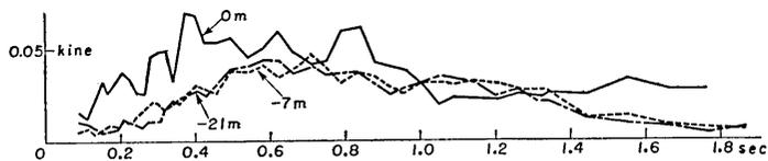
Fig. 85. Velocity spectra of earthquake No. 27 at place (B) in Tokai-mura.
