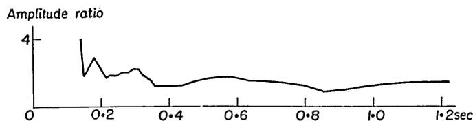
Fig. 8. Amplitude ratio of the ground surface to the 300 m depth at Hitachi Mine. Earthquake number: 441.
