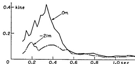
Fig. 53. Velocity spectra of earthquake No. 48 at place (A) in Tokai-mura.
