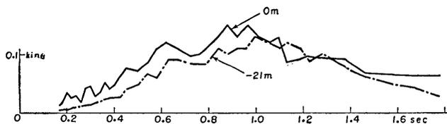
Fig. 47. Velocity spectra of earthquake No. 46 at place (A) in Tokai-mura.
