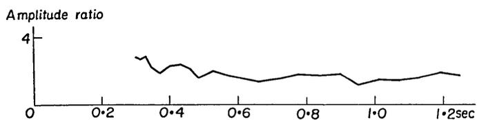
Fig. 7. Amplitude ratio of the ground surface to the 300 m depth at Hitachi Mine. Earthquake number: 428.
