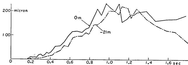
Fig. 38. Displacement spectra of earthquake No. 46 at place (A) in Tokai-mura.
