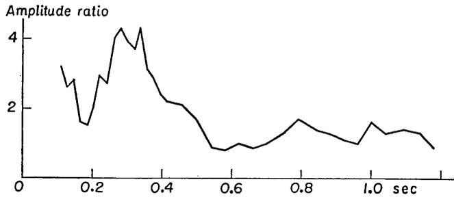
Fig. 71. The ratio of the amplitude on the ground to the one at 21 m depth at place (A) in Tokai-mura. Earthquake number: 48.
