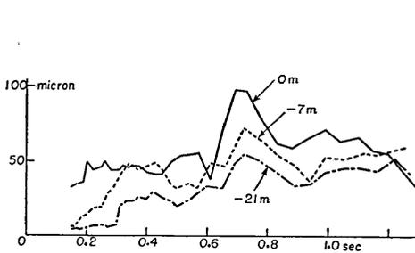
Fig. 72. Displacement spectra of earthquake No. 3 at place (B) in Tokai-mura.
