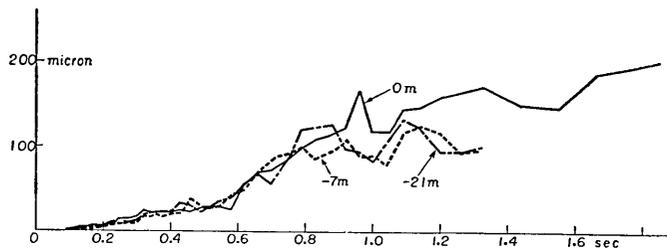
Fig. 77. Displacement spectra of earthquake No. 24 at place (B) in Tokai-mura.
