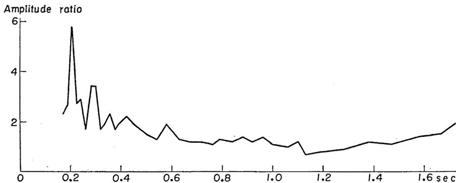
Fig. 65. The ratio of the amplitude on the ground to the one 21 m depth at place (A) in Tokai-mura. Earthquake number: 46.
