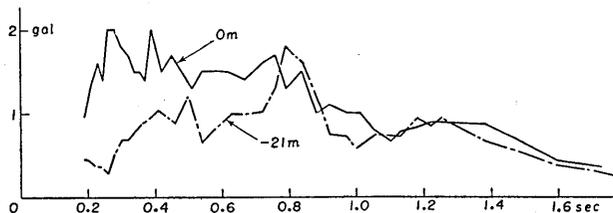
Fig. 57. Acceleration spectra of No. 50 earthquake at place (A) in Tokai-mura.
