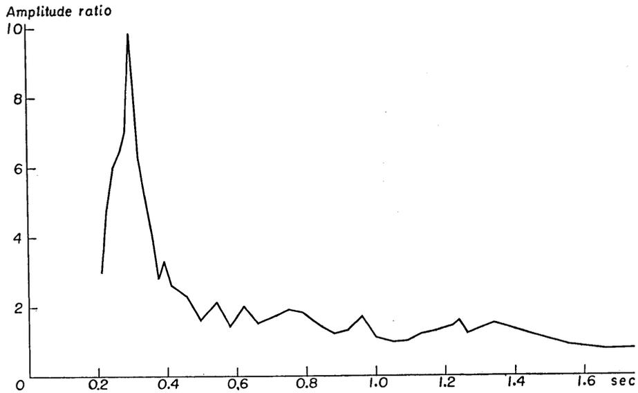
Fig. 69. The ratio of the amplitude on the ground to the one 21 m depth at place (A) in Tokai-mura. Earthquake number: 56.
