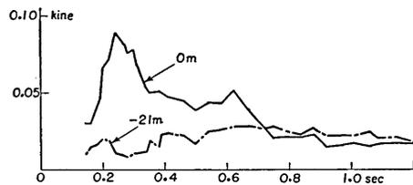
Fig. 46. Velocity spectra of earthquake No. 41 at place (A) in Tokai-mura.
