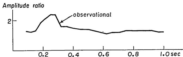
Fig. 104. Average amplitude ratio of -7 m to -21 m at place (B) in Tokai-mura.
