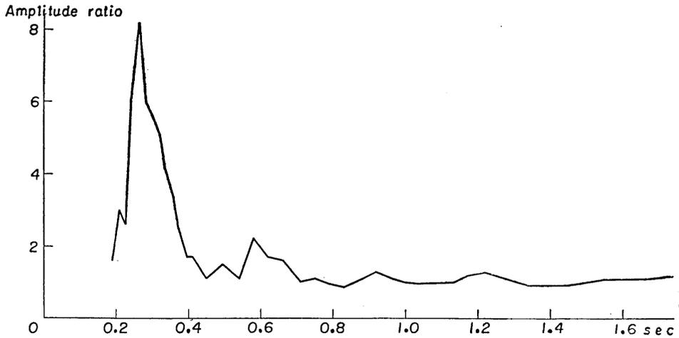
Fig. 67. The ratio of the amplitude on the ground to the one 21 m depth at place (A) in Tokai-mura. Earthquake number: 53.
