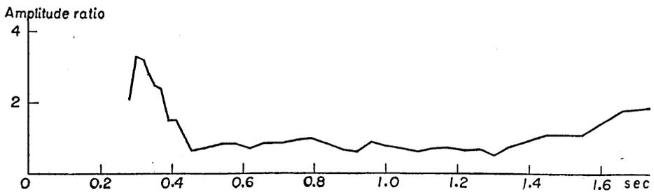
Fig. 68. The ratio of the amplitude on the ground to the one 21 m depth at place (A) in Tokai-mura. Earthquake number: 55.
