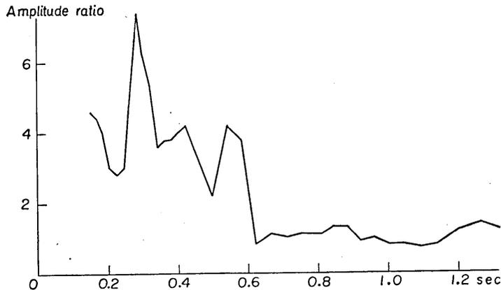
Fig. 63. The ratio of the amplitude on the ground to the one 21 m depth at place (A) in Tokai-mura. Earthquake number: 39.
