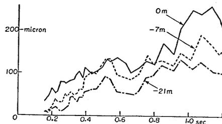
Fig. 75. Displacement spectra of earthquake No. 20 at place (B) in Tokai-mura.
