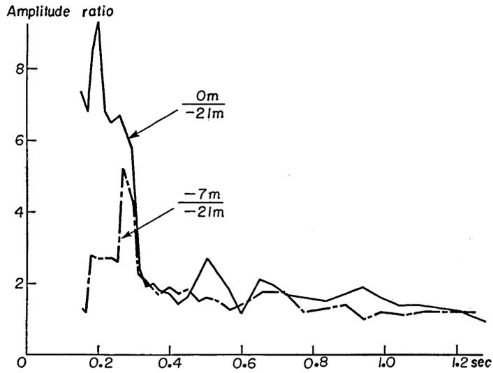
Fig. 93. Amplitude ratio corresponding to each period at place (B) in Tokai-mura. Earthquake number: 3.
