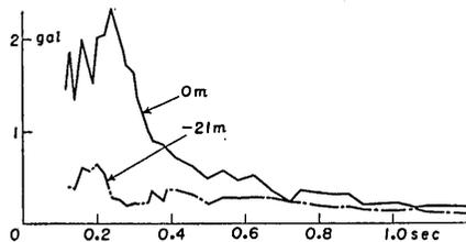
Fig. 55. Acceleration spectra of No. 41 earthquake at place (A) in Tokai-mura.
