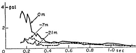
Fig. 88. Acceleration spectra of earthquake No. 10 at place (B) in Tokai-mura.
