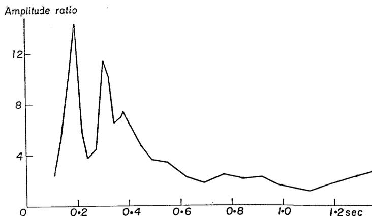
Fig. 5. Amplitude ratio of the ground surface to the 300 m depth at Hitachi Mine. Earthquake number: 200.
