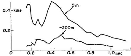
Fig. 23. Velocity spectra of earthquake No. 797 at Hitachi Mine.
