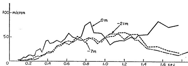
Fig. 78. Displacement spectra of earthquake No. 27 at place (B) in Tokai-mura.
