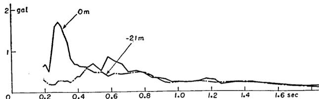
Fig. 58. Acceleration spectra of No. 53 earthquake at place (A) in Tokai-mura.
