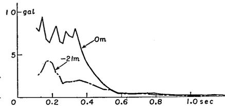
Fig. 62. Acceleration spectra of earthquake No. 48 at place (A) in Tokai-mura.
