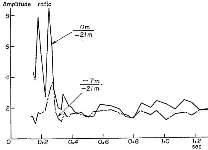
Fig. 97. Amplitude ratio corresponding to each period at place (B) in Tokai-mura. Earthquake number: 20.
