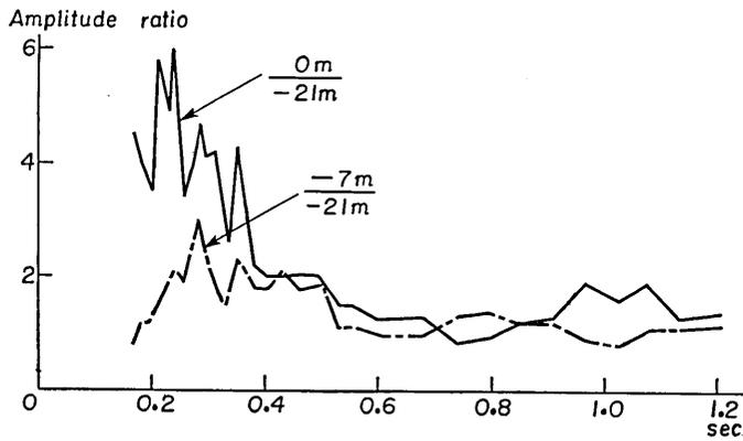
Fig. 95. Amplitude ratio corresponding to each period at place (B) in Tokai-mura. Earthquake number: 10.
