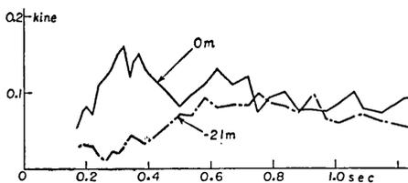
Fig. 52. Velocity spectra of earthquake No. 63 at place (A) in Tokai-mura.
