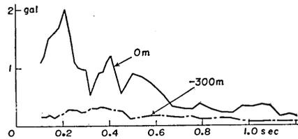
Fig. 31. Acceleration spectra of earthquake No. 828 at Hitachi Mine.
