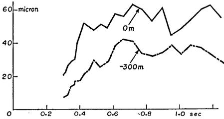
Fig. 14. Displacement spectra of earthquake No. 428 at Hitachi Mine.
