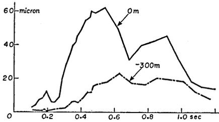
Fig. 12. Displacement spectra of earthquake No. 200 at Hitachi Mine.
