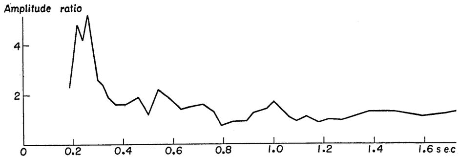
Fig. 66. The ratio of the amplitude on the ground to the one 21 m depth at place (A) in Tokai-mura. Earthquake number: 50.
