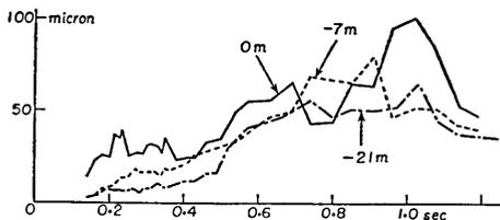
Fig. 74. Displacement spectra of earthquake No. 10 at place (B) in Tokai-mura.
