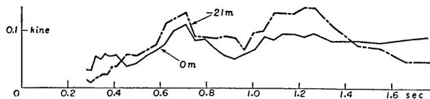
Fig. 50. Velocity spectra of earthquake No. 55 at place (A) in Tokai-mura.
