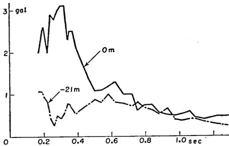
Fig. 61. Acceleration spectra of earthquake No. 63 at place (A) in Tokai-mura
