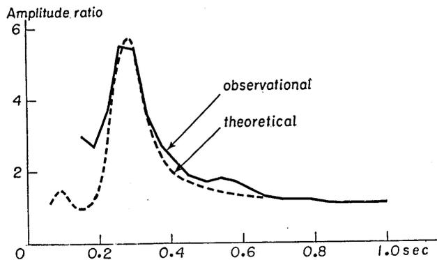
Fig. 102. Average amplitude ratio of 0 m to -21 m at place (A) in Tokai-mura.
