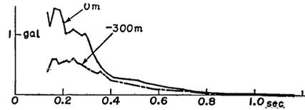
Fig. 29. Acceleration spectra of earthquake No. 441 at Hitachi Mine.
