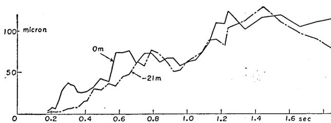
Fig. 40. Displacement spectra of earthquake No. 53 at place (A) in Tokai-mura.
