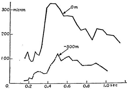
Fig. 16. Displacement spectra of earthquake No. 797 at Hitachi Mine.
