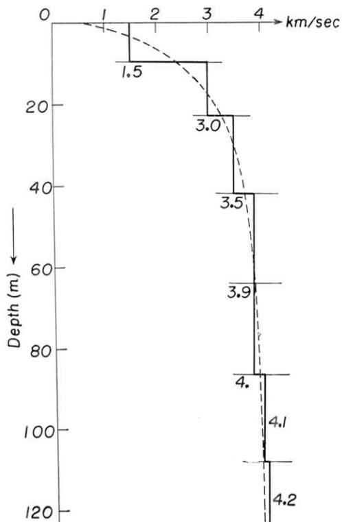
Fig. 2. Velocity of *P*-waves versus depth from the earth's surface at Hitachi Mine.
