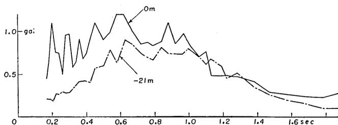
Fig. 56. Acceleration spectra of No. 46 earthquake at place (A) in Tokai-mura.
