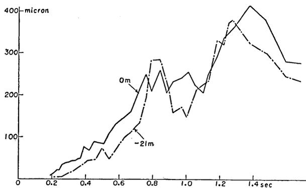
Fig. 39. Displacement spectra of earthquake No. 50 at place (A) in Tokai-mura.
