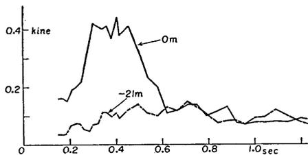
Fig. 45. Velocity spectra of earthquake No. 39 at place (A) in Tokai-mura.
