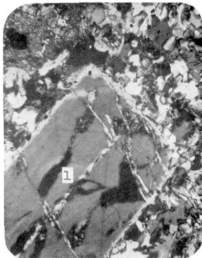
Fig. 9. Trachytic andesite (Fukazawa-fudō). The texture of groundmass resembles that of plagioliparite, but is quite free of quartz phenocrysts. 1=Plagioclase. \times 100 .
