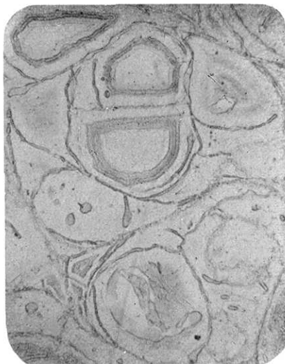
Fig. 7. Perlite (The cutting of the bus road between Iwanoshita and Sugarita). \times 100 .
