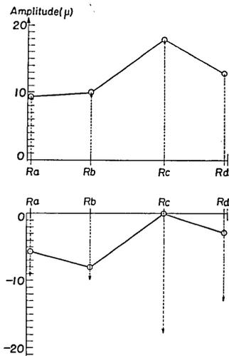
Fig. 22 b. Horizontal amplitude distributions at the moments within 1/4 cycle of vibration, including the moment when the amplitude of position *Rc* (roof-floor) of No. 6 house became maximum.
