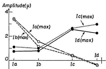
Fig. 21 b. Amplitude distributions at the moment when the horizontal amplitude of each position at the first-floor of No. 6 house became maximum.
