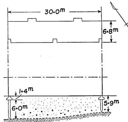
Fig. 5. Sketch of the foundation parts of No. 14 house.
