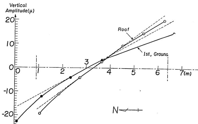
Fig. 11. Distributions of resonance amplitudes of vertical component of No. 14 house.
