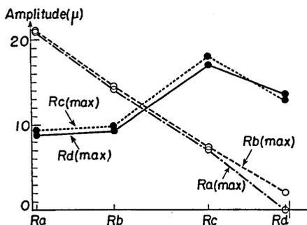
Fig. 21 a. Amplitude distributions at the moment when the horizontal amplitude of each position at the roof-floor of No. 6 house became maximum.
