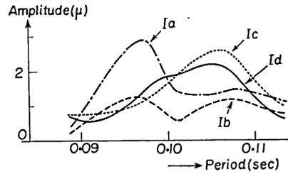
Fig. 17b. Amplitude-period relations at first-floor of No. 6 house.
