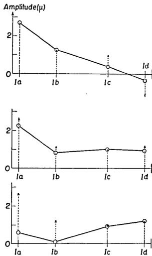
Fig. 22 c. Horizontal amplitude distributions at the moments within 1/4 cycle of vibration, including the moment when the amplitude of position *Ib* (first-floor) of No. 6 house became maximum.
