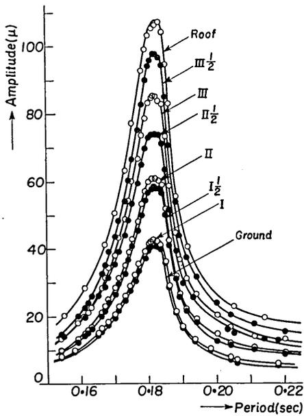
Fig. 7. Amplitude-period relations of horizontal component of No. 14 house.
