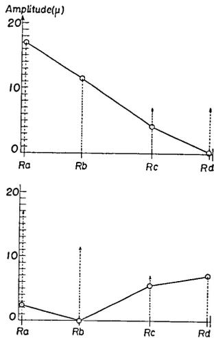
Fig. 22 a. Horizontal amplitude distributions at the moments within 1/4 cycle of vibration, including the moment when the amplitude of position *Rb* (roof-floor) of No. 6 house became maximum.
