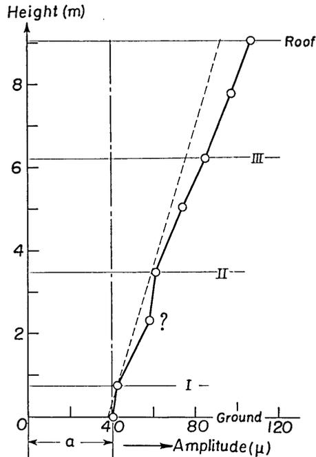
Fig. 8. Amplitude distribution of horizontal component of No. 14 house.
