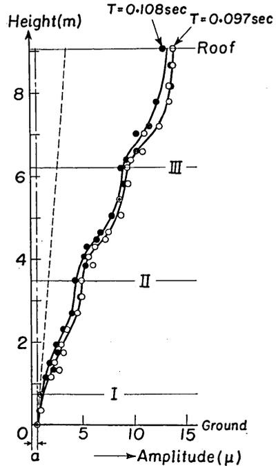
Fig. 19. Amplitude distributions of horizontal component of No. 6 house.
