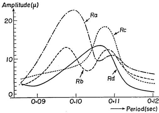
Fig. 17a. Amplitude-period relations at roof-floor of No. 6 house.
