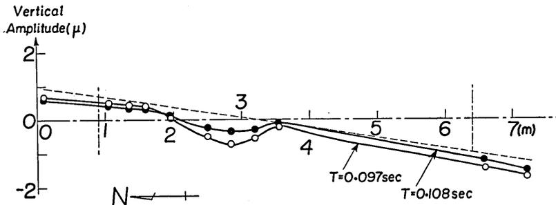
Fig. 20b. Amplitude distributions of vertical component at first-floor of No. 6 house.
