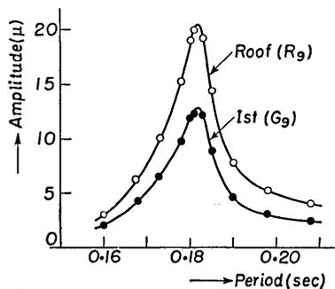
Fig. 10. Amplitude-period relations of vertical component of No. 14 house.
