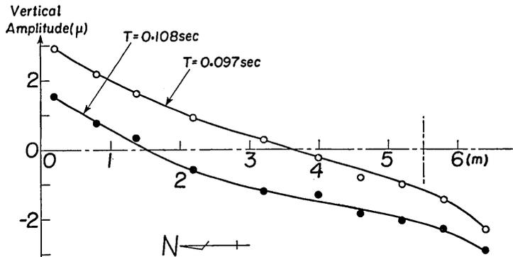
Fig. 20a. Amplitude distributions of vertical component at roof-floor of No. 6 house.
