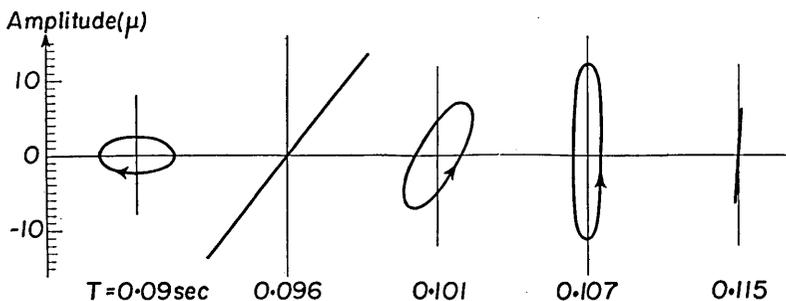
Fig. 24. Horizontal orbital motions at  $R_e$  (roof-floor) of No. 6 house.
