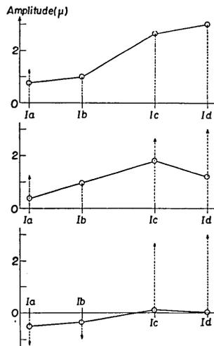
Fig. 22 d. Horizontal amplitude distributions at the moments within 1/4 cycle of vibration, including the moment when the amplitude of position *Ic* (first-floor) of No. 6 house became maximum.
