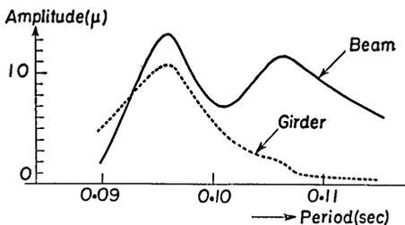
Fig. 23. Amplitude-period relation of both the beam and girder directions of No. 6 house observed simultaneously.
