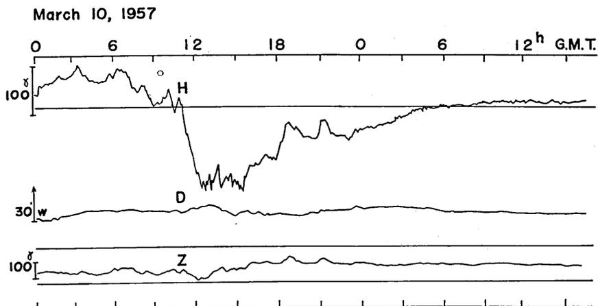
Fig. 6 The magnetogram obtained at Aburatsubo station. The magnetic storm occurred at 0h 21m GMT on March 10, 1957.
