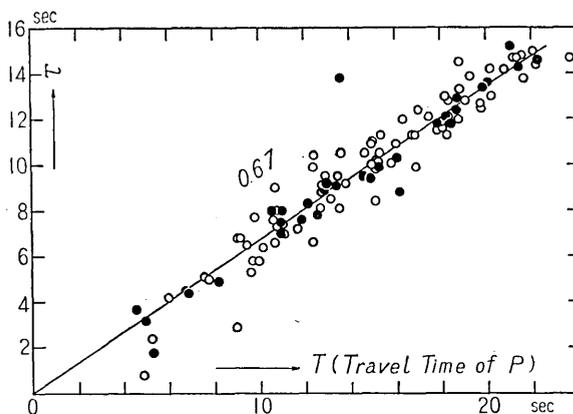
Fig. 1.  $T$  (Travel time of P)  $\sim$   $\tau$  (P-S interval) relation of the earthquakes in the Kinki district, origin time of P being assumed at the time when  $\tau=0$ . And  $\bullet$  Earthq. No. 5, 6, 8;  $\circ$  Earthq. No. 9~14.
