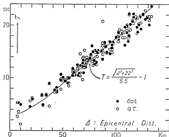
Fig. 3. Time-distance relation of the earthquakes No. 5, 6, 8, 9, 10, 11, 12 and 14.
