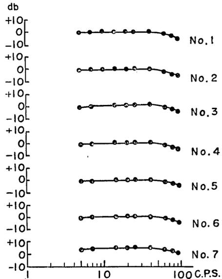
Fig. 8-b. Over-all frequency characteristics.
