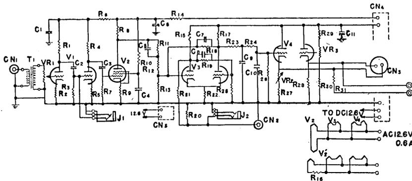
Fig. 4-c. Circuit diagram of demodulator.
