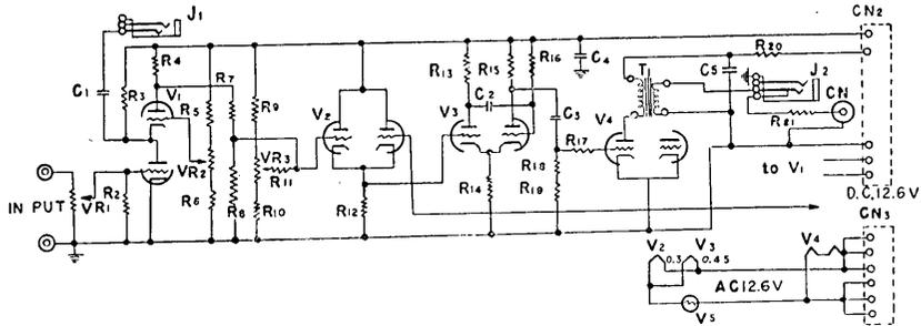
Fig. 4-a. Circuit diagrams of amplifier and modulator.
