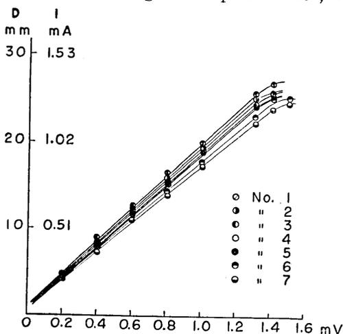
Fig. 9. Relation between the input voltage and the recorded amplitude of different channels at a fixed cycle, 14 cps.
