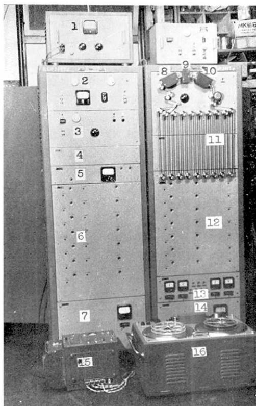
Fig. 2. 1. Preamplifier. 2. Power controller 3. Recording time controller. 4. Trigger unit. 5. Level meter. 6. D.C. Amplifier and modulator. 7. Power unit. 8. Playback head. 9. Erasing head. 10. Recording head. 11. Endless tape. 12. Demodulator. 13. Output meter. 14. Power unit. 15. Recording oscillograph. 16. Preservation magnetic tape recorder.
