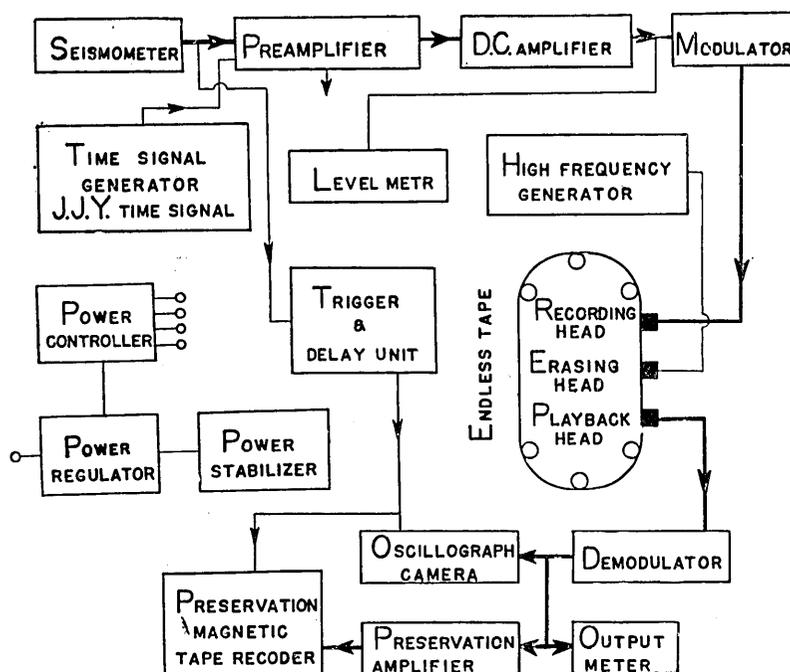
Fig. 1. Block diagrams of the equipment.
