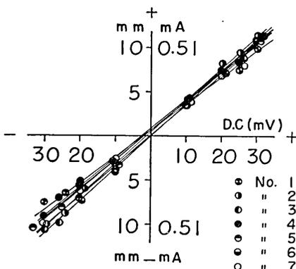
Fig. 3. Characteristic curves of direct-coupled amplifier, that indicate input voltage and output current relations.
