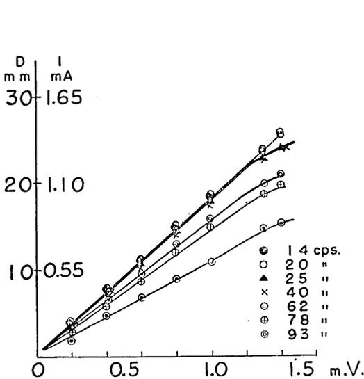
Fig. 8-a. The relation between the input voltage and the recorded amplitude with respect to different frequencies.
