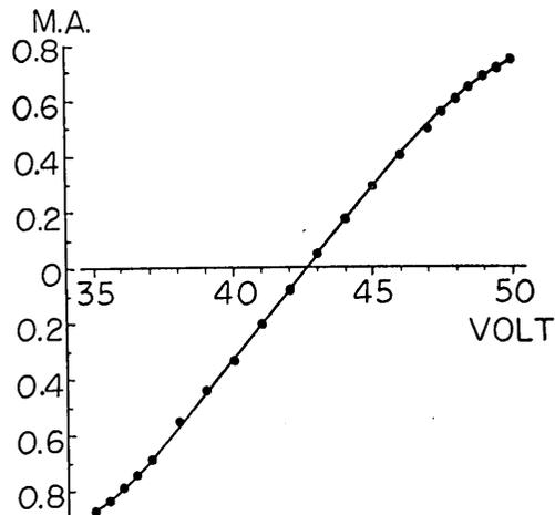
Fig. 5. Modulation and demodulation characteristic curve of a channel. Abscissa is an input voltage to a modulator. Ordinate is the output current from a demodulator. (In this figure the modulator and the demodulator are connected directly, without passing through the magnetic tape.)
