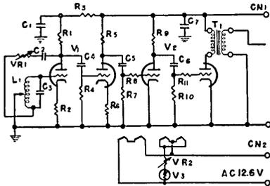
Fig. 4-b. Circuit diagram of pulse generator.
