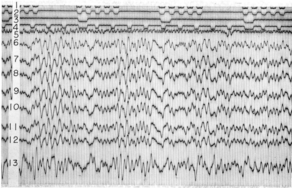
Fig. 10-b. An example of a record of the ground noise. The output voltage from a seismometer is fed in parallel to the seven channels of the magnetic tape recorder. (2/3 the actual)
