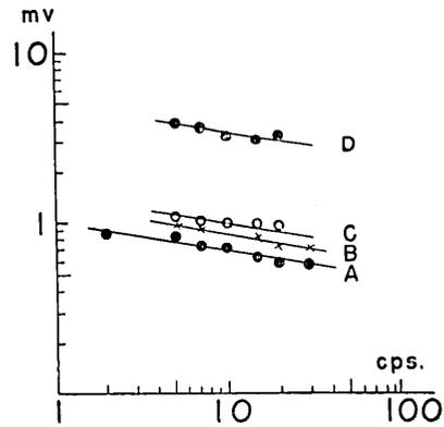
Fig. 7. Diagram indicating the trigger level. Indicator points the graduation D; No. 4, C; No. 6, B; No. 8, A; No. 10 (maximum sensitivity).
