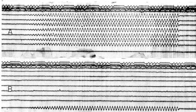
Fig. 10-a. Fidelity test record of the tape recorder system. An alternating voltage is applied in parallel to the seismometer terminal of respective seven channel. (1/4 the actual)
