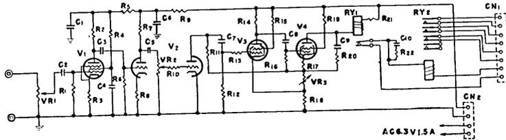
Fig. 6. Trigger circuit diagram.
