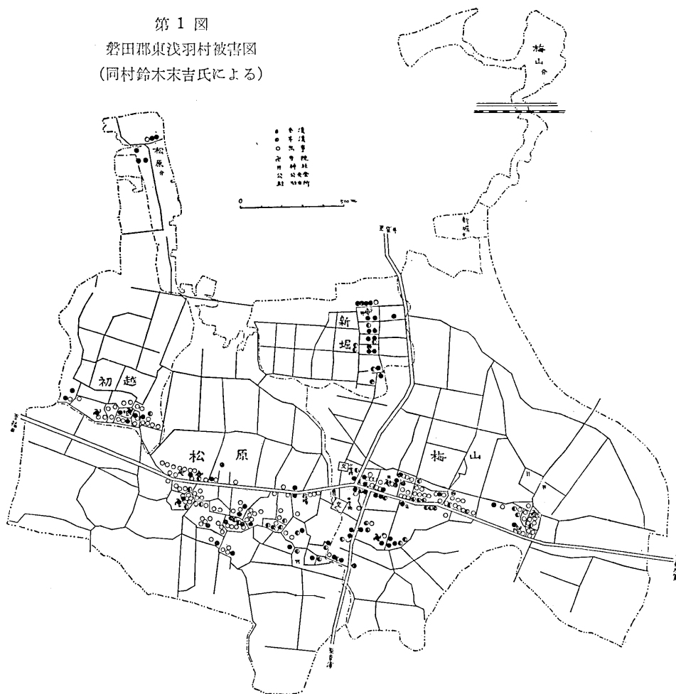
Fig. 1. Distribution of damaged houses in Higashi-Asaba Village, Iwata County. Black and half-black circles denote the totally collapsed and half collapsed dwelling houses, respectively, while circles denote undamaged ones.
