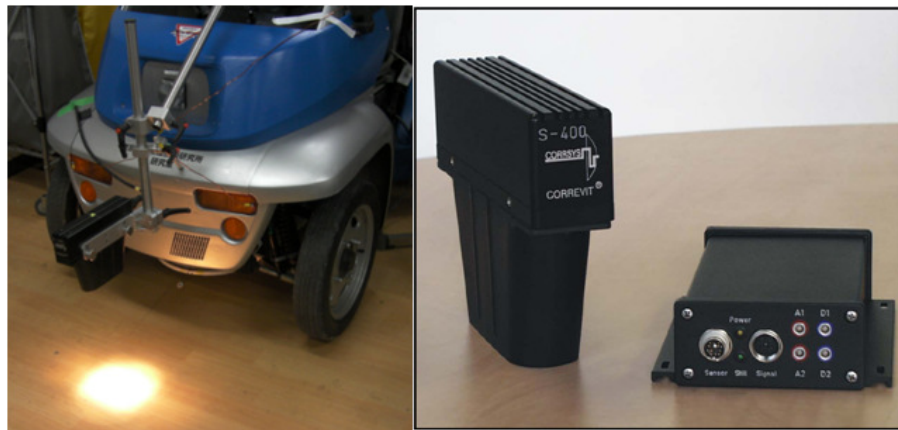
Fig 1.4 Corsys-Datron optical sensor for sideslip angle measurement
