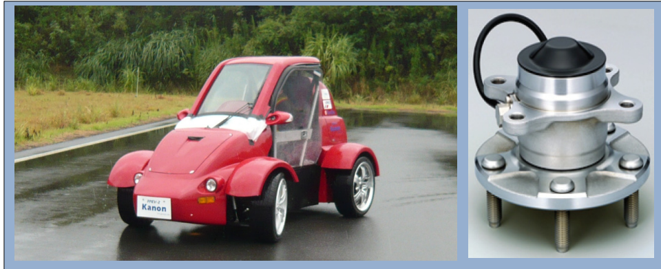
Fig. 1 Experimental electric vehicle Kanon and tire lateral force sensor
