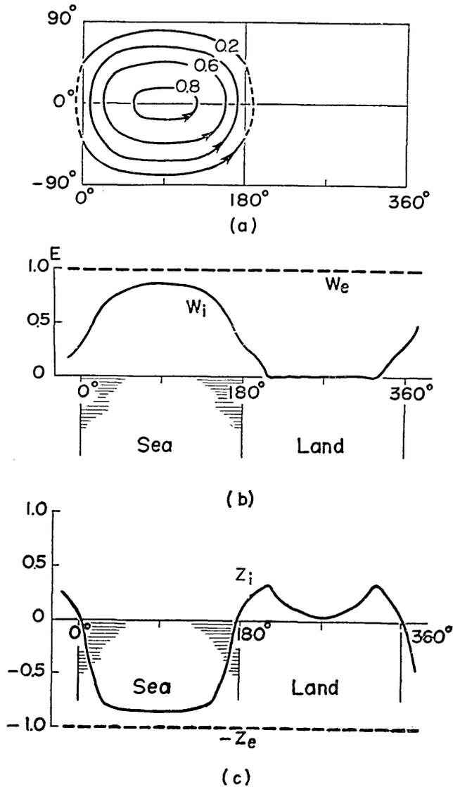
Fig 14. (a) The induced electric currents at  $t=0$ . (b) The distribution of the inducing and induced magnetic potential or current function on  $y=0$ . (c) The same distribution of the vertical component of the inducing and induced fields. (Unit:  $\frac{\pi}{a}E$ )
