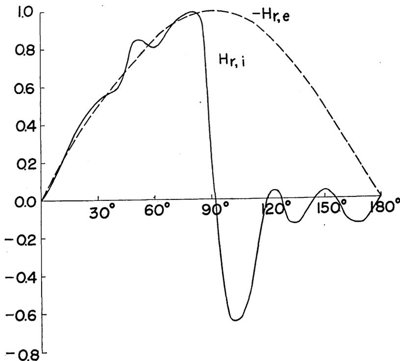
Fig. 11. The initial distribution of the normal component of the inducing and induced magnetic field on  $\phi = 0$ . (Unit:  $H_0$ )
