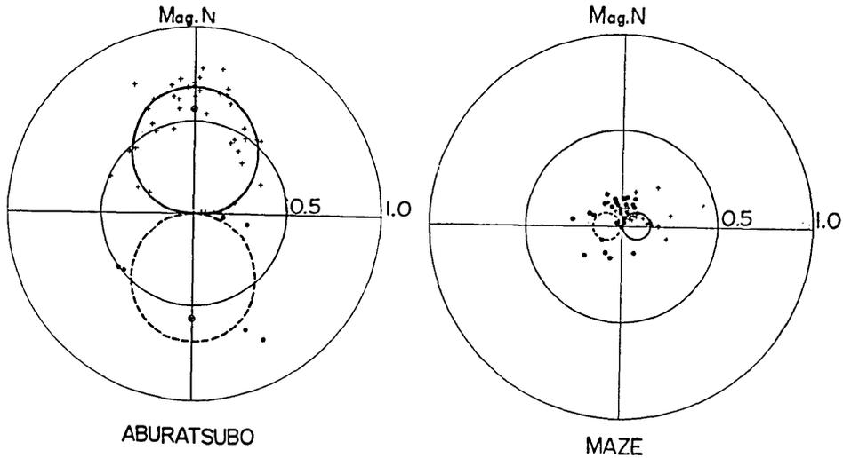
Fig. 6a. The relation between  $\Delta Z/\Delta R$  and the direction of the magnetic vector in the horizontal plane at Aburatsubo. Fig. 6b. The relation between  $\Delta Z/\Delta R$  and the direction of the magnetic vector in the horizontal plane at Maze.
