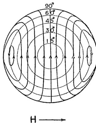
Fig. 10. The distribution of the initial currents, the same amount of the electric current flowing between two adjacent lines.
