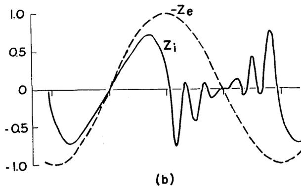
Fig. 13. (a) The inducing and induced magnetic potential or current function. (b) The vertical component of the inducing and induced field. (Unit:  $\frac{\pi}{a} E$ )
