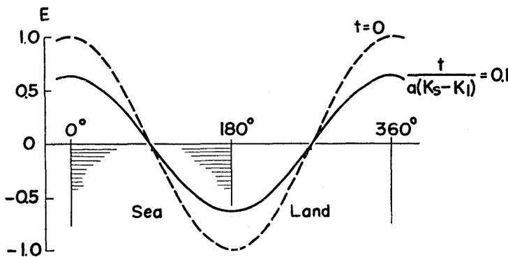
Fig. 16. The distribution of the induced (broken line) magnetic potential or current function at  $t=0$ , while that at  $t=1$  sec. is shown by the full line. The conductivities are taken to be  $2 \times 10^{-7}$  and  $10^{-7}$  emu respectively and  $a$  is assumed to be  $10^8$  cm.
