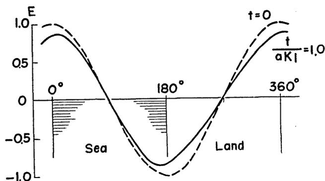
Fig. 15. The induced (broken line) magnetic potential or current function at  $t=0$ , while that at  $t=0.1$  sec. is shown by the full line. The conductivity on the sea is taken to be infinity, while that on the land is assumed to be  $10^{-9}$  emu and  $a$  to be  $10^8$  cm.
