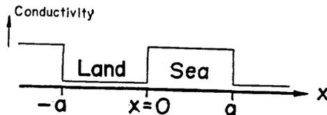
Fig. 12. The supposed distribution of the electrical conductivity on the land and sea.
