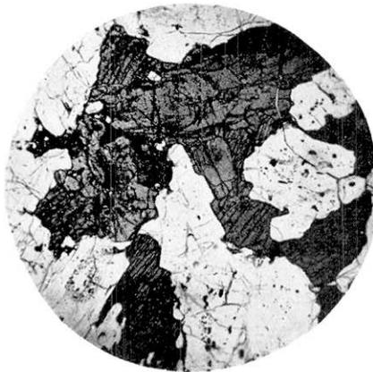
Fig. 28. Magnetite-olivine-hypersthene-augite-plagioclase-rock (isolated ejecta).  $\times 15$ .
