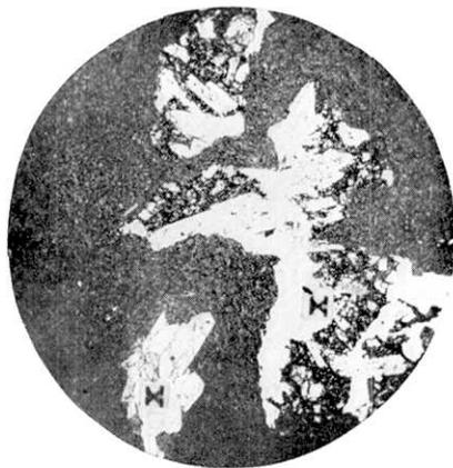
Fig. 23. Microphotograph of the obsidian (Fig. 22)  $\times 15$ . x: xenolith (augite-plagioclase-rock). x': xenolith (olivine-basalt).
