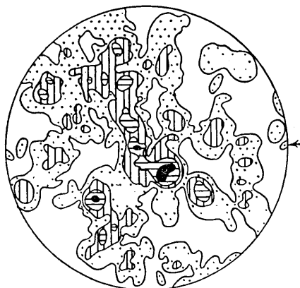
Fig. 4, Orientation diagram for c axes of calcite in specimen III. 211 grains per diagram. Contours, 0~1, 1~2, 2~4, 4~5%, per 1% area.
