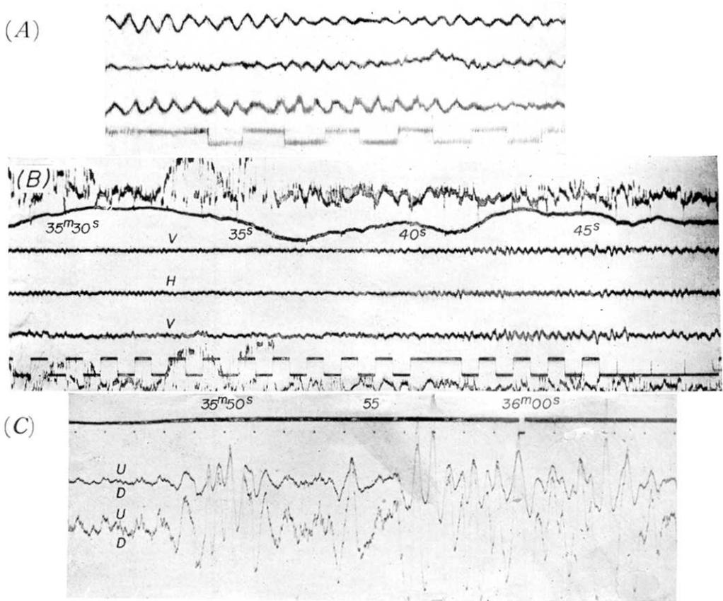
Fig. 6. Seismograms obtained at the first Kamaisi explosion of 1952 on the southern profile at Siroiwa (A), Nogizawa (B) and Hitati (C).
