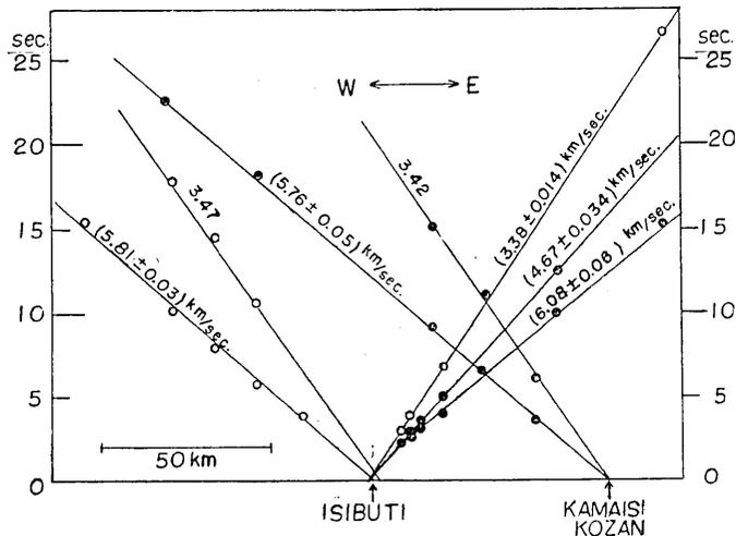
Fig. 3. Time-distance curves of the E-W profile of the first Kamaisi explosion seismic observations.
