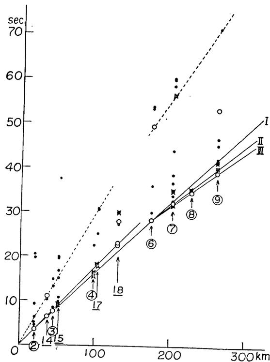
Fig. 2. Time-distance curves in the southern profile of the first Kamaisi explosion seismic observations.
