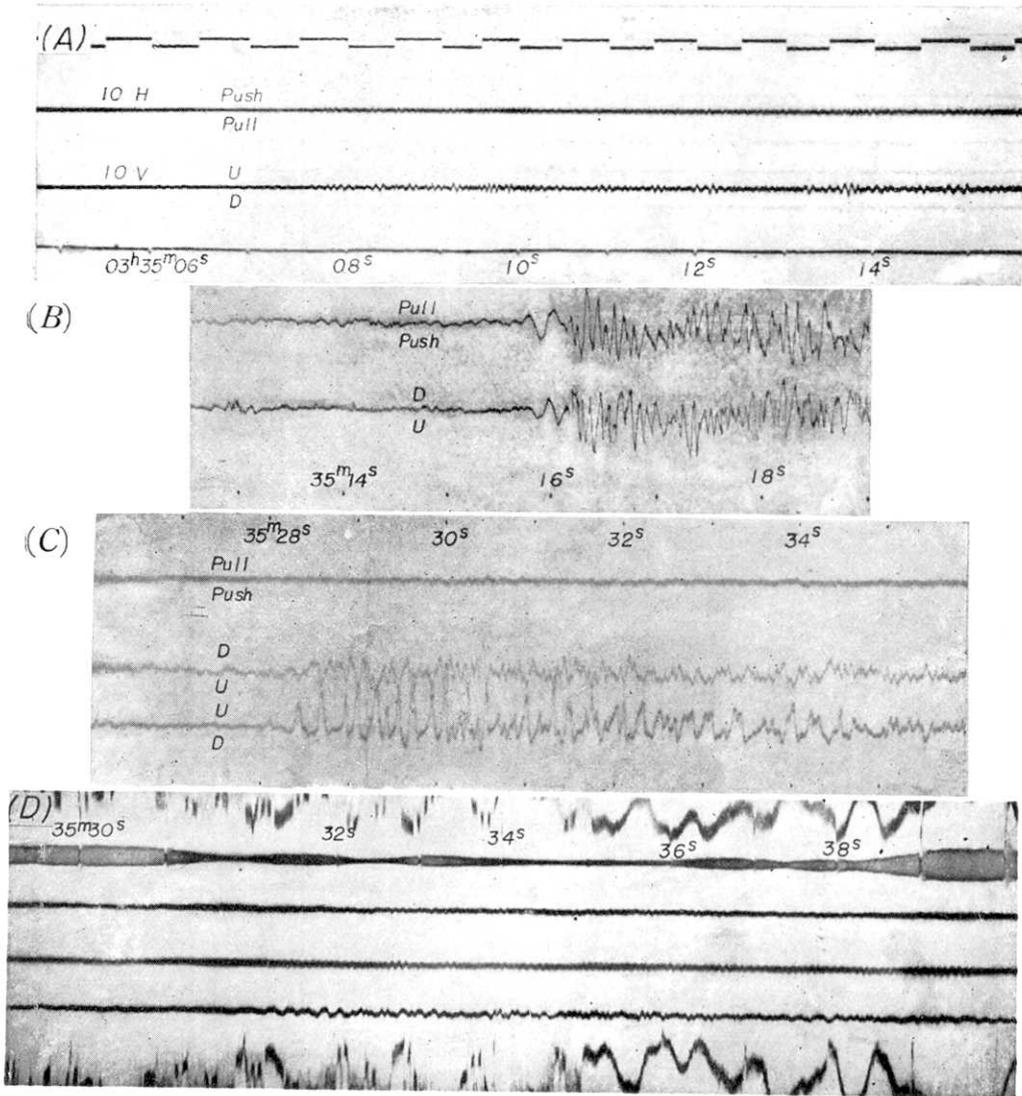
Fig. 5. Seismograms obtained at the first Kamaisi explosion of 1952 on the southern profile at Kesennuma (A), Onagawa (B), Kanayama (C) and Kawamata (D).
