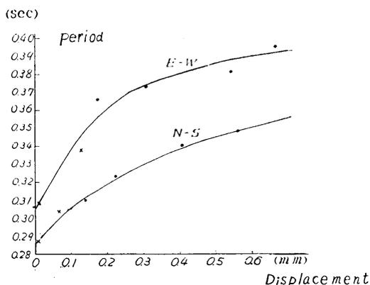
Fig. 14. Relation between displacement amplitude and resonance period.
