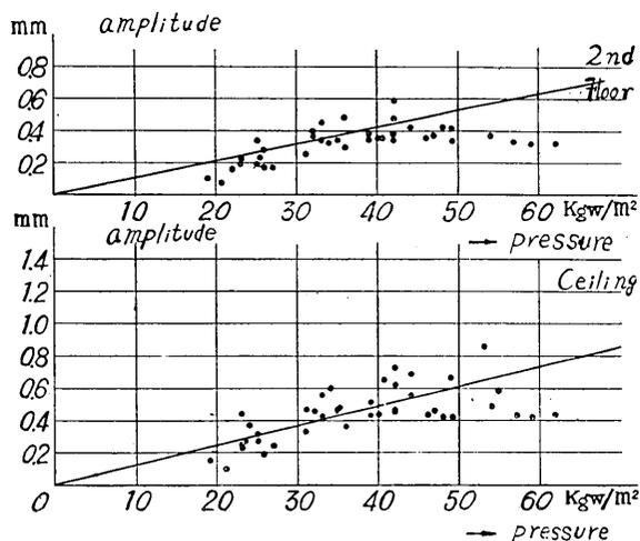
Fig. 16. Relation between wind pressure and house displacement amplitude S-W wind.
