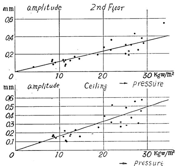
Fig. 15. Relation between wind pressure and house displacement amplitude S-W wind.
