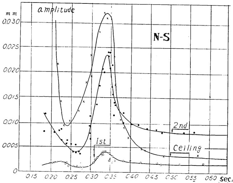
Fig. 9. Relations between displacement amplitude and period.
