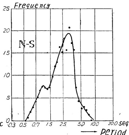
Fig. 20. Relation between vibration period of the house due to N-E wind and their predominant period. Observation time=17<sup>h</sup>40<sup>m</sup>~17<sup>h</sup>45<sup>m</sup>, March 2, 1941.
