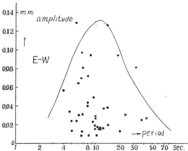
Fig. 27. Relation between vibration amplitude and period due to S-W wind.
