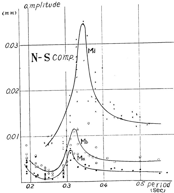
Fig. 11b. Vibration characteristics of the 2nd floor for the variation of unbalanced mass of the rotary.
