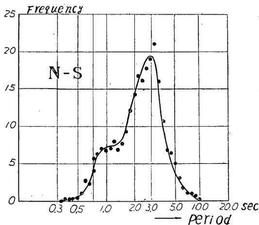
Fig. 19. Relation between vibration period of the house due to N-E wind and their predominant period. Observation time=17<sup>h</sup>35<sup>m</sup>~17<sup>h</sup>40<sup>m</sup>, March 2, 1941.
