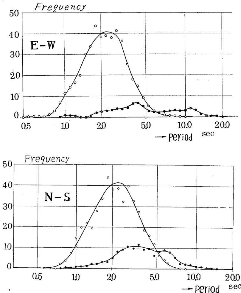
Fig. 23. Vibration period of the house due to S-W wind and their predominant period. 12<sup>h</sup>17<sup>m</sup> to 12<sup>h</sup>27<sup>m</sup>.
