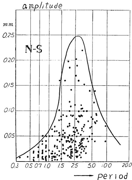
Fig. 24. Vibration period and amplitude (N-S comp.) due to E-N wind.
