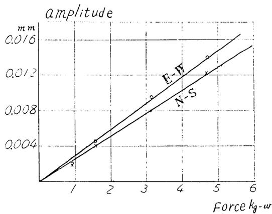
Fig. 12. Relation between the applied statical force and the maximum horizontal deflection of the 2nd floor.
