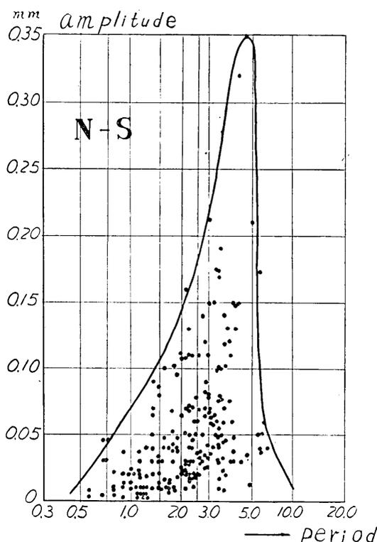
Fig. 25. Vibration period and amplitude (N-S comp.) due to E-N wind.
