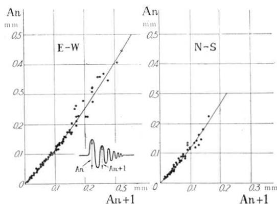
Fig. 5. Damping characters of E-W, N-S component free vibrations on the 2nd floor.
