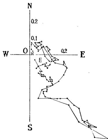
Fig. 28. Vector diagram of the house vibration due to the wind during about 60 sec. from 2<sup>h</sup>45<sup>m</sup>40<sup>s</sup> on March 4, 1941.
