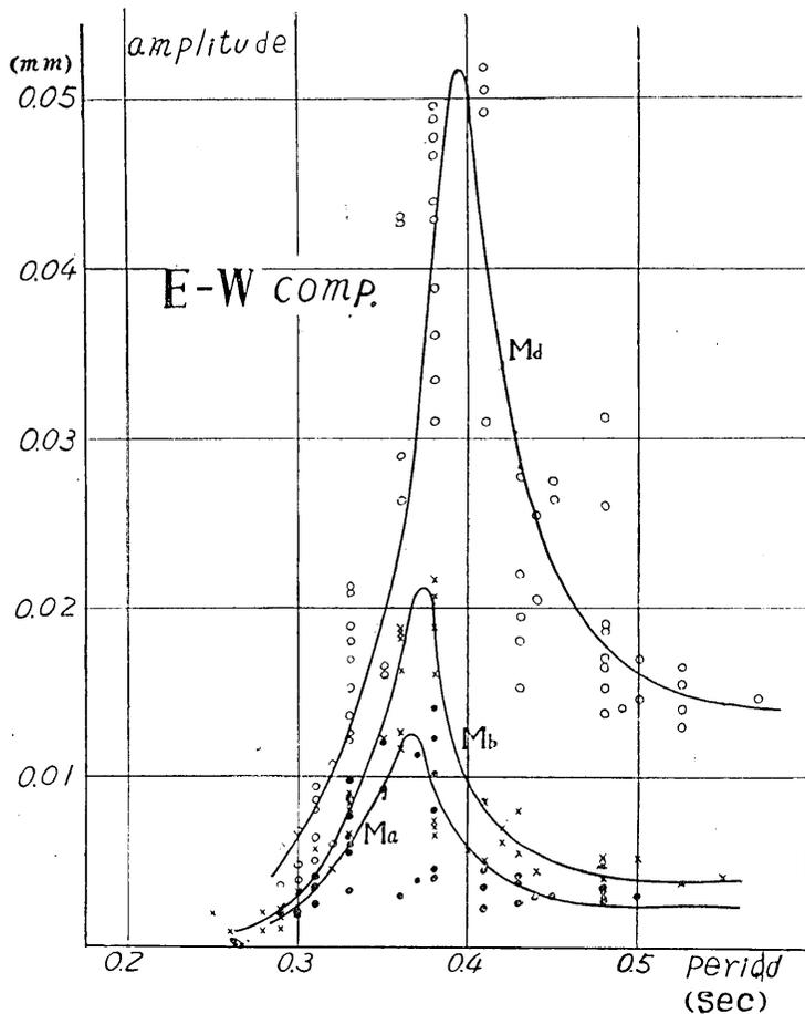
Fig. 11a. Vibration characteristics of the 2nd floor for the variation of unbalanced mass of the rotary.
