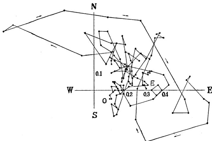
Fig. 29. Vector diagram of the house vibration due to the wind during about 50 sec. from 2<sup>h</sup>45<sup>m</sup> 0<sup>s</sup> on March 4, 1941.
