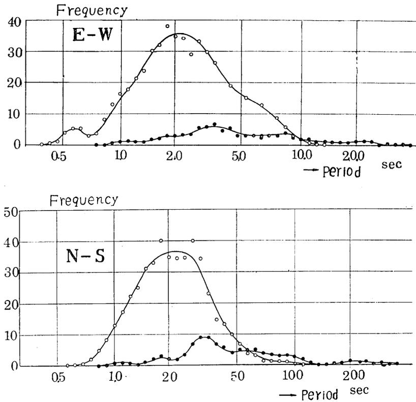
Fig. 22. Relation between vibration period of the house due to N-E wind and their predominant period. 17<sup>h</sup>45<sup>m</sup> to 17<sup>h</sup>55<sup>m</sup> March 2, 1941.
