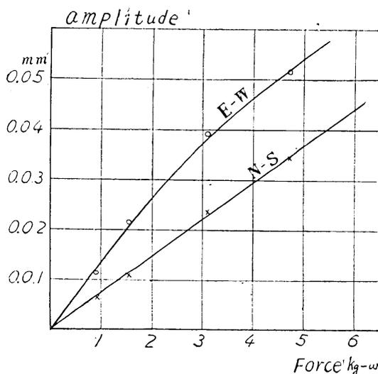
Fig. 13. Relation between applied dynamical force and maximum deflection at 2nd floor.
