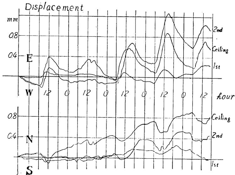
Fig. 30. Displacement of the house due to the sun's radiation heat.
