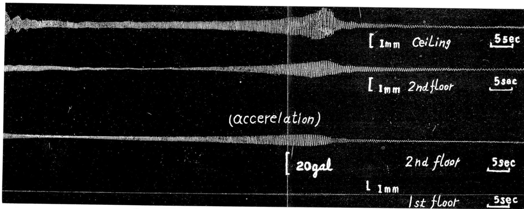
Fig. 8. E-W comp. records of the forced vibrations. Unbalanced mass  $M_c=3.4$  kg.
