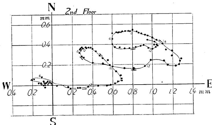
Fig. 31. Vector diagram of the house due to the sun's radiation heat.
