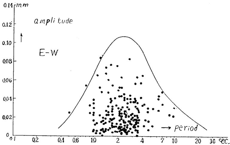
Fig. 26. Relation between vibration amplitudes and period due to S-W wind.
