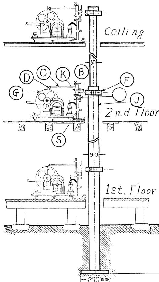
Fig. 3a. Measuring apparatus for house deformation.
