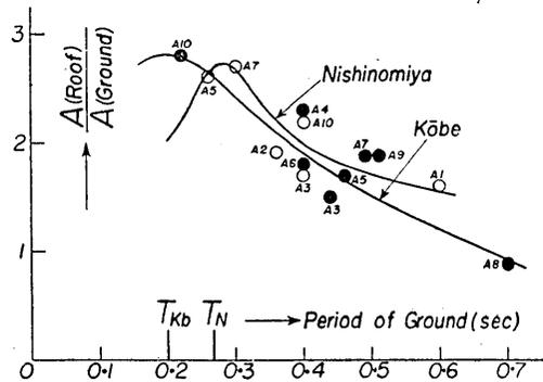
Fig. 27.  $A$  and  $T$  represent the largest amplitude and the natural period of building respectively.
