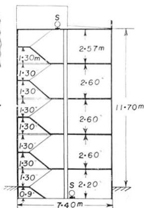
Fig. 1b. Side view of type 49B.
