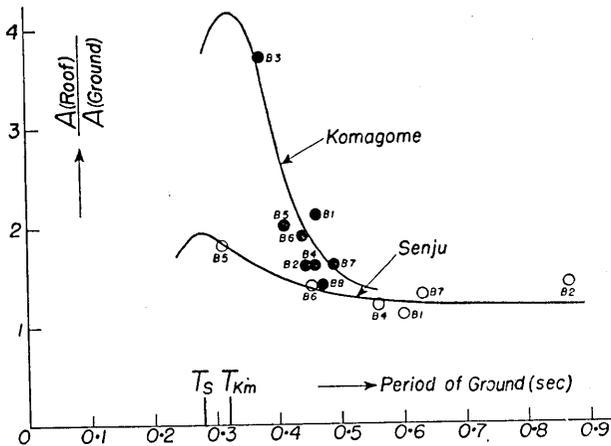
Fig. 28.  $A$  and  $T$  represent the largest amplitude and the natural period of building respectively.
