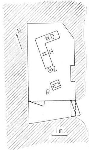
Fig. 2. The arrangement of the *D* (declination)-, *H* (horizontal-intensity)-, and *Z* (vertical intensity)-magnetometers and *R* (recording drum) in the magnetometer room.
