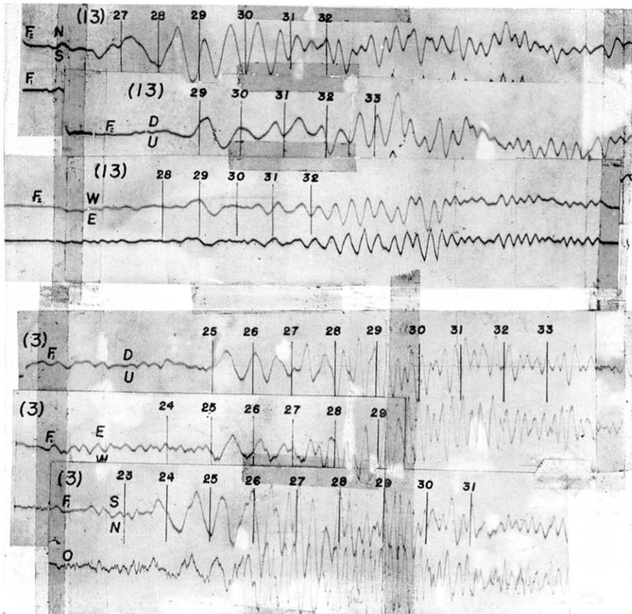
Fig. 3. Examples of the filtered record representing the separated Love and Rayleigh waves.
