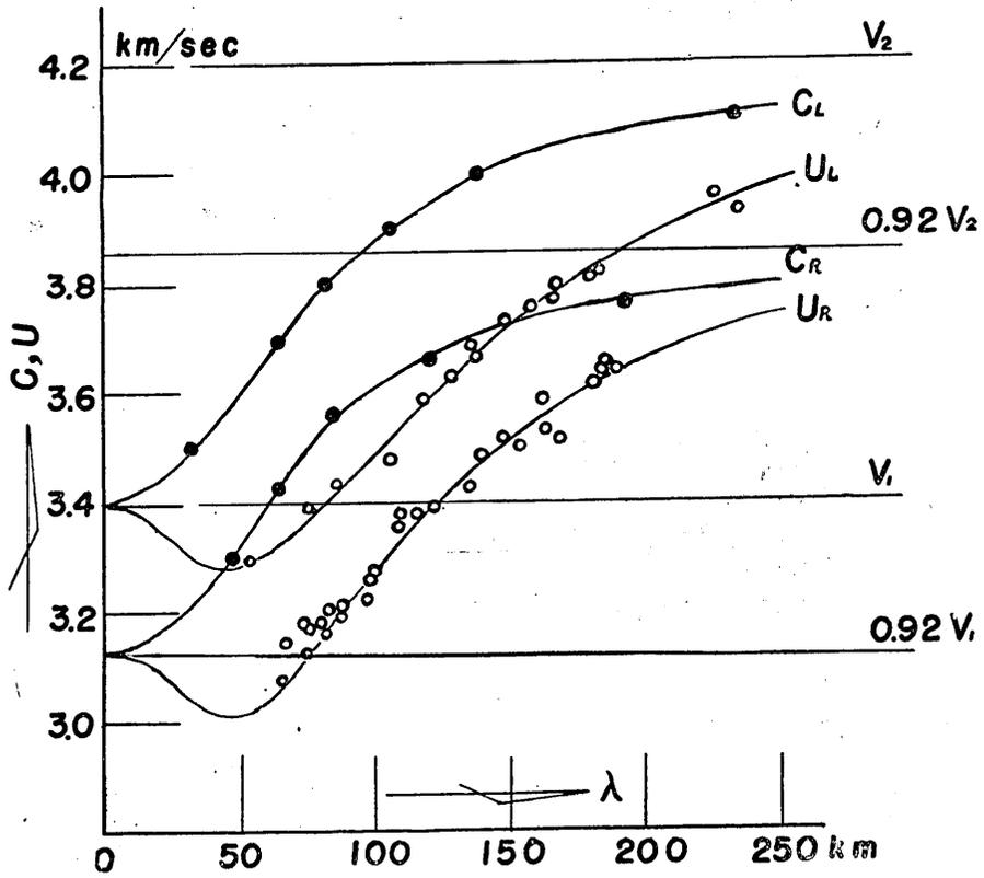
Fig. 13. The estimated crustal structure of (c) region and the results of theoretical calculations (filled circle).
