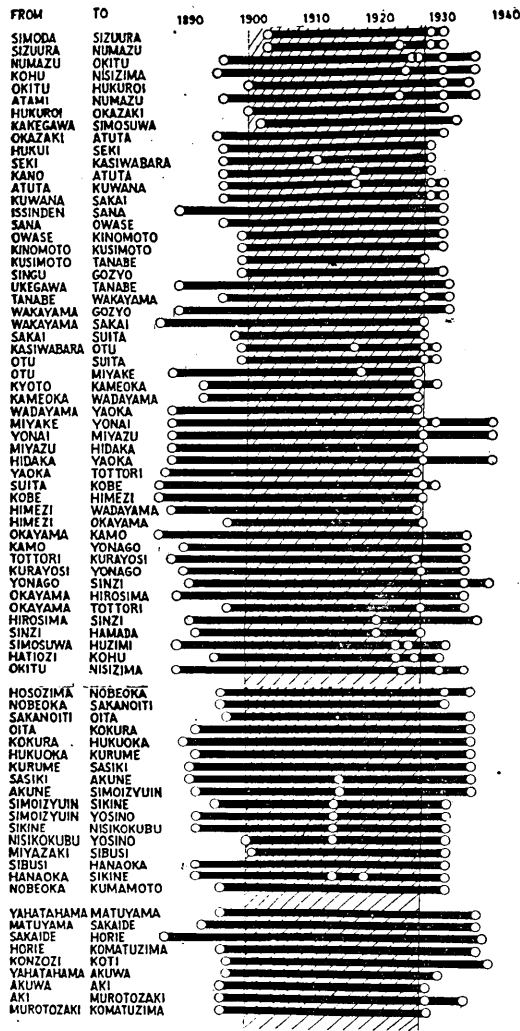
Fig. 2b. Dates of Surveys for Lines of Levels. (Circles designate the epochs of surveys)
