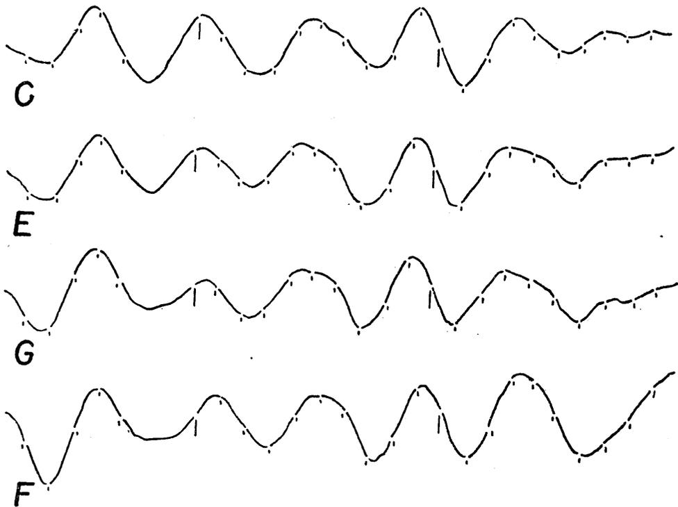
Fig. 1(a). Microseisms, September 11, 1950, 11<sup>h</sup> 18<sup>m</sup>, observed at *C*-, *E*-, *G*-, and *F*-stations, respectively. Interval between time marks is one second.
