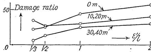
Fig. 2. The relation among the damage ratio, ground condition and  $\epsilon'/l$  for the case of ferro-concrete buildings in the former Tokyo city at the time of the Kwanto earthquake of 1923. 0m.....40m represent the thickness of alluvium.
