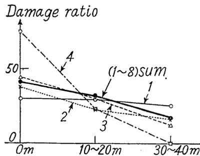
Fig. 4. The relation between the damage ratio and the thickness of alluvium for the case of ferro-concrete buildings in the former Tokyo city at the time of the Kwanto earthquake of 1923. 1, 2, .... represent the number of stories.
