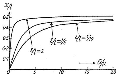
Fig. 7. The results of mathematical calculations of the relation between height where stress take maximum and ratio of  $G/\mu$ .
