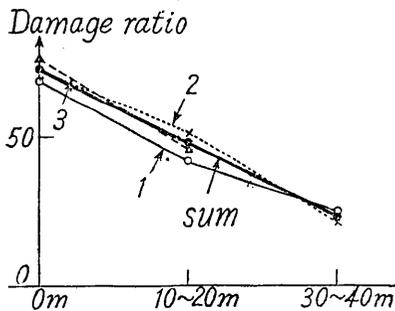
Fig. 3. The relation between the damage ratio and thickness of alluvium for the case of brick buildings in the former Tokyo city at the time of the Kwanto earthquake of 1923. 1, 2, 3 represent the number of stories.
