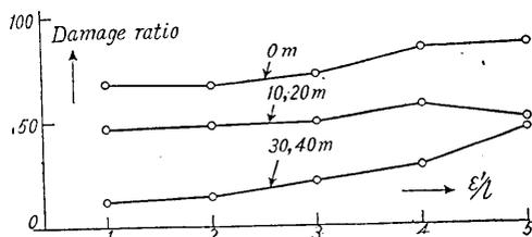
Fig. 1. The relation among the damage ratio, ground condition and  $\epsilon'/l$  for the case of brick buildings in the former Tokyo city at the time of the Kwanto earthquake of 1923. 0m...40m represent the thickness of alluvium.
