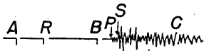
Fig. 2. An example of a seismograph with time marks. R is radio mark A, B and C are minute marks.
