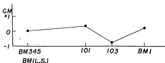
Fig. 8. Change in the altitude difference of BM 1 compared with the BM 345 of the Land Survey.
