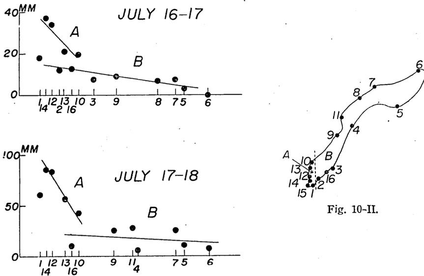
Fig. 10-I. Tilting of ground revealed by the survey of Pond-4. Location of dots corresponding to respective figures in Fig.10-I are seen in the map of Fig. 10-II. The amount of tilt in the A-part is definitely larger than the B-part.
