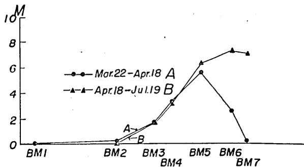
Fig. 2. Changes in the altitude difference of bench marks.
