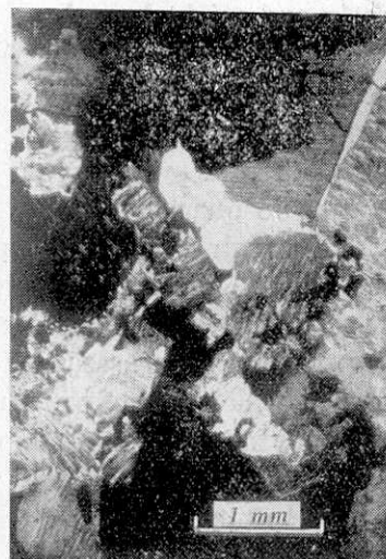
Fig. 6. Micropertthitic felspar forming the principal portion of the quartz-syenite exposed along the road side west of Isa. Microphoto., analyzer being inserted.
