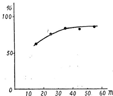
Fig. 4. Relation between thickness of alluvium and damage rate in the A-plain.
