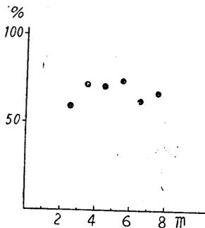
Fig. 7. Relations between the damage rate and thickness of reclaimed mud in the A-plain,
