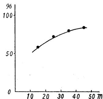
Fig. 5. Relation between thickness of alluvium and damage rate in the B-plain.
