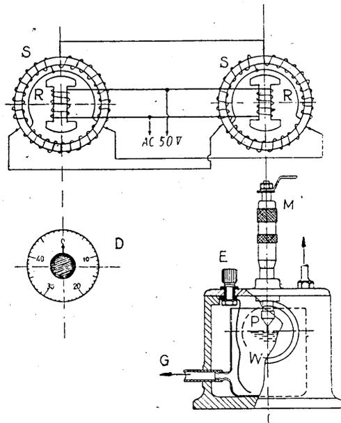
Fig. 4. The schematic view of the main part of the water-tube tiltmeter and the circuit for self-synchronous motors.
