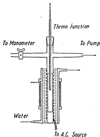
Fig. 2. Non-magnetic and non-inductive vacuum furnace in the apparatus.
