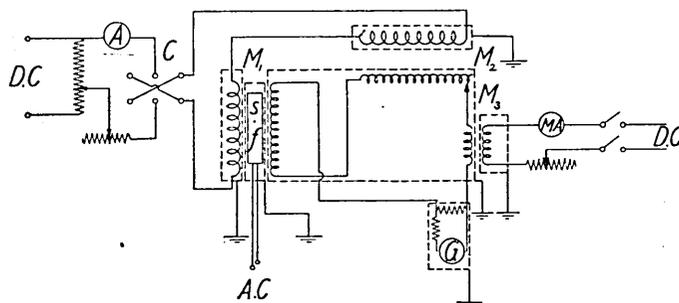
Fig. 1. Electric circuit in the apparatus for measuring susceptibility at high temperature.
