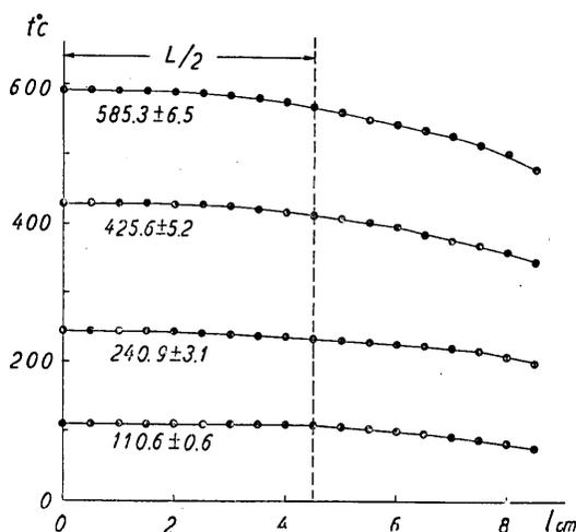
Fig. 4. Temperature distribution in the furnace.  $L$  denotes the length of specimen. (Heating velocity = 2 degree/min.)
