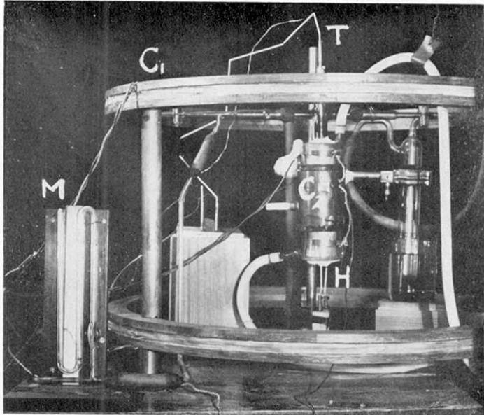
Fig. 3 a. Apparatus for measuring the magnetic susceptibility at high temperature.
