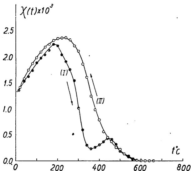
Fig. 11. Change in magnetic susceptibility with temperature (irreversible type). No. 7 (S-N 59)  $H=2.20$  gauss.
