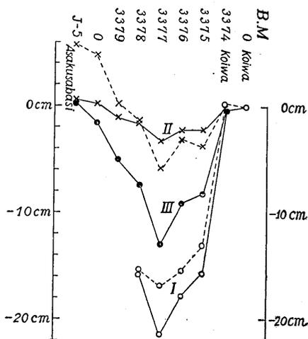
Fig. 2. Corrected (full lines) and uncorrected (dotted lines) vertical displacements of bench-marks along the line between Koiwa and Asakusabasi.
