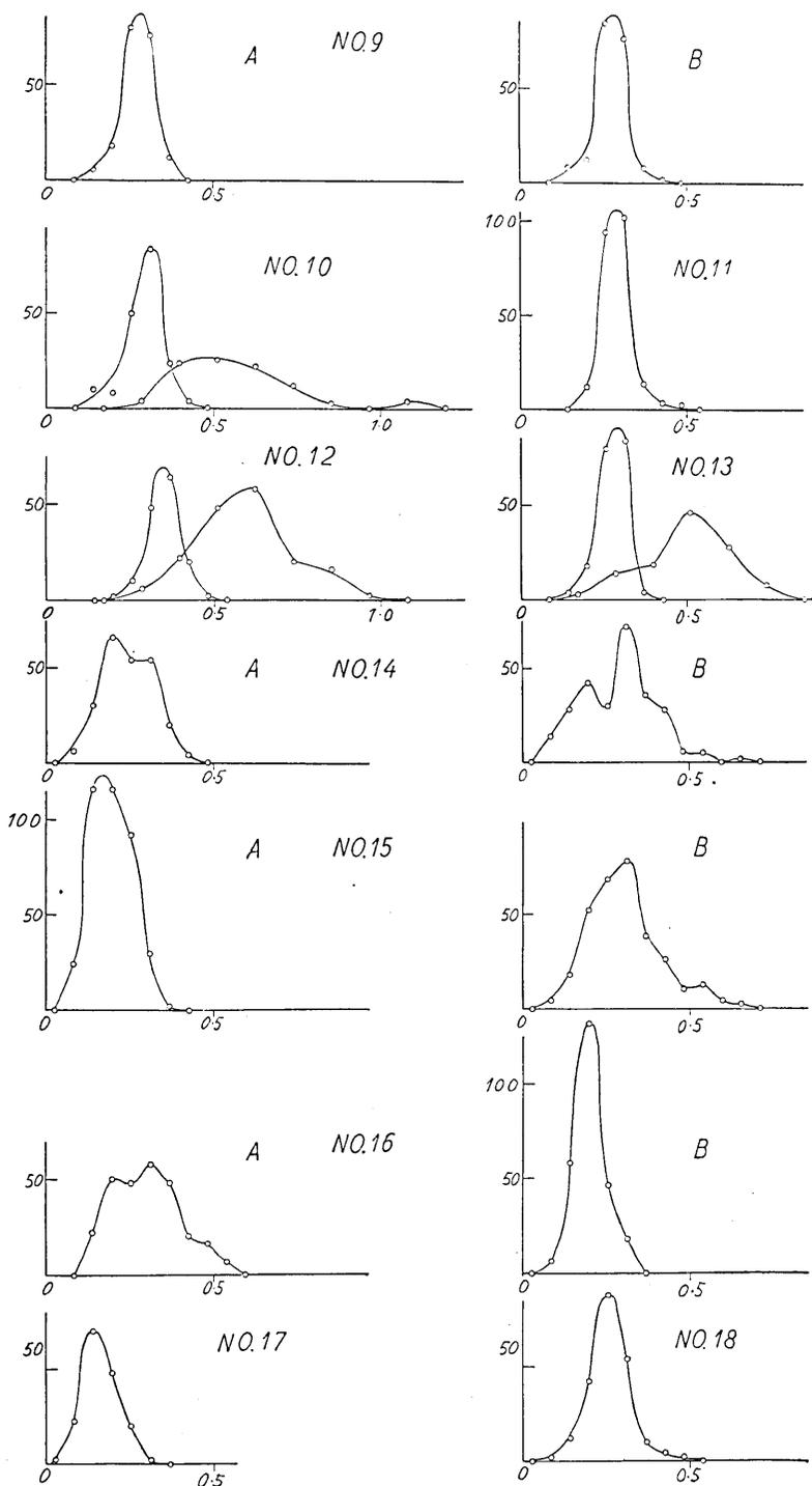
Fig. 6b. Frequency curves of the periods of tremors observed at the various stations. B. The component in the direction of the crater. A. The component that is perpendicular to B.
