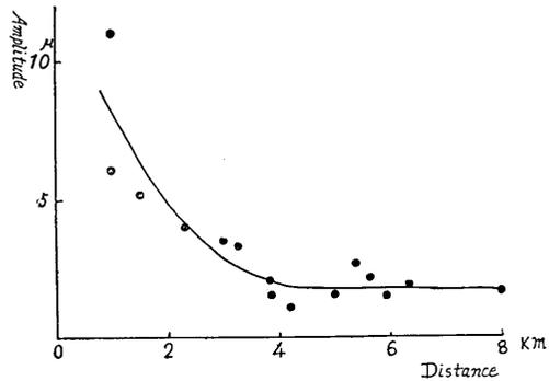
Fig. 12. Decrease in amplitude with increasing distance from the crater.
