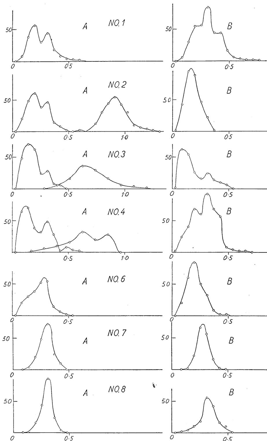
Fig. 6a. Frequency curves of the periods of tremors observed at the various stations. B. The component in the direction of the crater. A. The component that is perpendicular to B.
