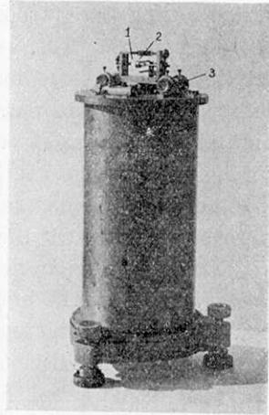
Fig. 1. Seismograph used in the present measurements.
