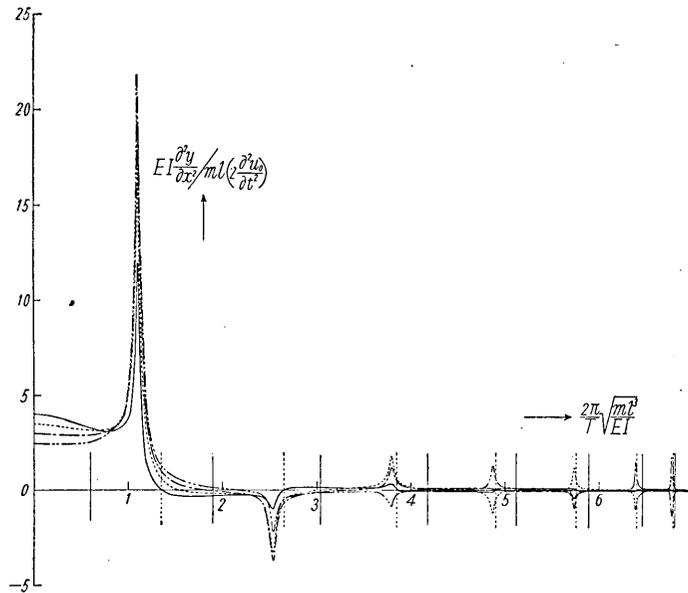
Fig. 3 a. Full, broken, chain, and double chain lines represent moments in columns of ground, first, second, and third floors respectively.
