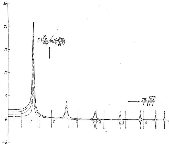
Fig. 3 b. Full, broken, chain, and double chain lines represent moments in columns of fourth, fifth, sixth, and seventh floors respectively.
