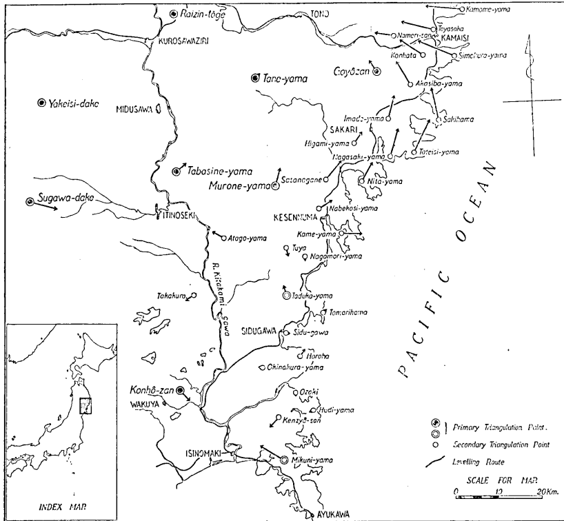
Fig. 1. Distribution of triangulation points and level lines. (Arrows show the horizontal displacements of the triangulation points.)
