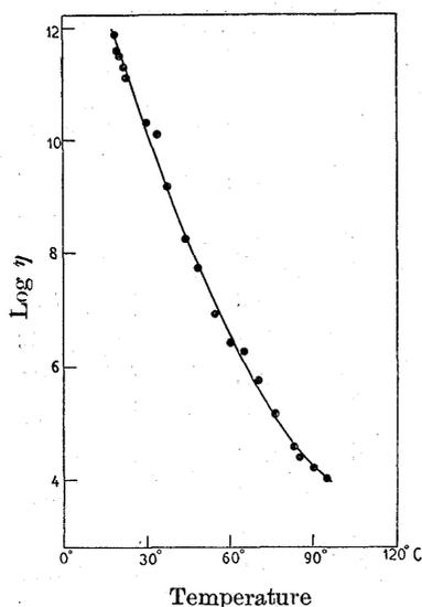
Fig. 10. Curve of temperature and the log. of viscosity coefficient of pitch.
