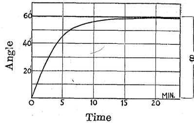
Fig. 7. Relaxation curve of twisted water-glass. The straight line shows the twisted constant angle  $\varphi=59'$
