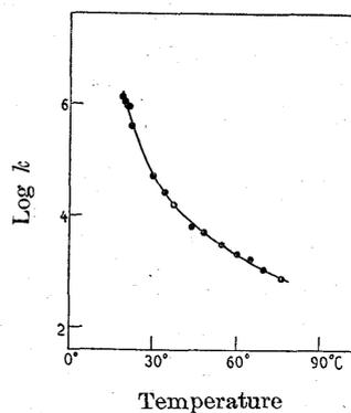
Fig. 13. Curve of temperature and the log. of apparent rigidity of pitch.
