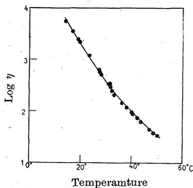
Fig. 12. Curve of temperature and the log. of viscosity coefficient of water-glass.
