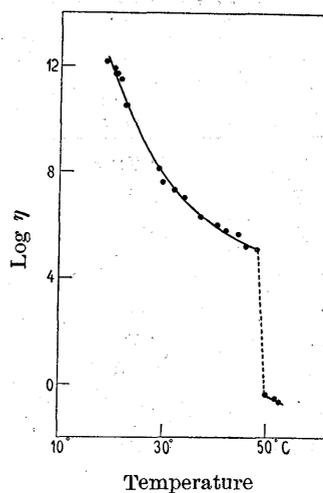
Fig. 11. Curve of temperature and the log. of viscosity coefficient of Paraffin.
