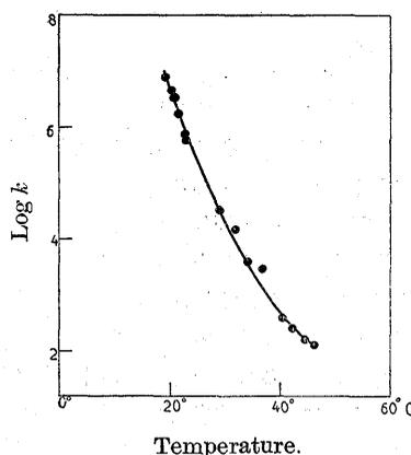
Fig. 14. Curve of temperature and the log. of apparent rigidity of paraffin.
