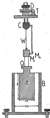
Fig. 9. Concentric cylinder apparatus.
