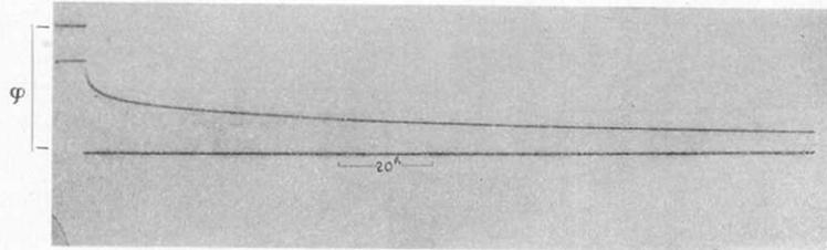
Fig. 3. Record of twisted paraffin cylinder (No. 2).
