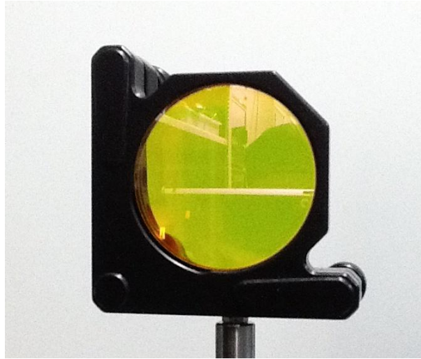
Fig.2.7 Collecting lens (ZnSe-lens)
